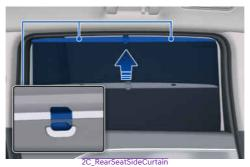
Use the rear side sunshade to block the light coming through the rear seat windows. Lift the rear side sunshade and hang the sunshade on both sides of the hook.
