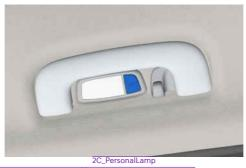
স: Press the button to turn on and off the rear room lamp.
