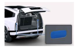
The cargo area lamp comes on when the liftgate is opened.
