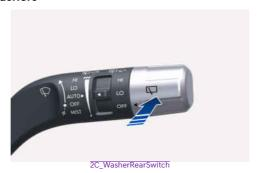
Push the lever away from you to spray rear washer fluid and to run the rear wipers 1-3 cycles. The spray and wiper operation continues until you release the lever.
