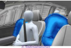
Side airbags are located in the outboard of front and rear seats. Additionally, a front center side airbag is located in the inboard side of the driver seatback.
