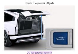
Press the power liftgate open/close button to open/close the liftgate with a warning sounds.
