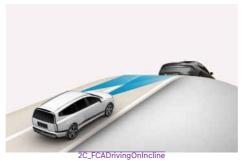
During uphill or downhill driving, the SCC may not detect a moving vehicle in your lane, and cause your vehicle to accelerate to the set speed. Also, vehicle speed rapidly decreases when the vehicle ahead is detected suddenly. Select the appropriate set
