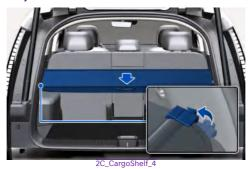
Pull the cargo security screen towards the rear of the vehicle and insert the guide pin into the guide.
