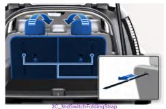
· When using it as a seat, pull the seatback angle adjustment strap to fully raise the seatback. Adjust the seatback to the desired angle, and release the upper angle adjustment strap to lock in place. Make sure the seatback is locked in place.
