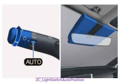
The headlights and parking lights are turned ON or OFF automatically depending on the amount of daylight as measured by the ambient light sensor in front of the instrument panel.
