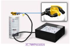
3. Unscrew the valve cap from the valve of the defective wheel and screw the filling hose of the sealant bottle onto the tire valve.
