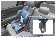
3. Check the Child Restraint System is secure by pushing and pulling the seat forward and back and side-to-side.
