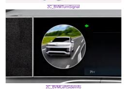
When the left or right side turn signal turns on, the image in that direction appears on the instrument cluster.
