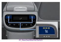
While the vehicle is running, press the seat warmer button to warm the rear seat.
