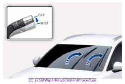
Within 20 seconds of turning off the vehicle, lift and hold the wiper lever up to the MIST position for about 2 seconds until the wipers move to the top wipe position.
