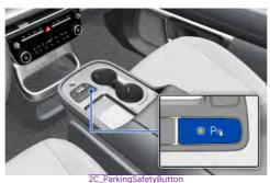
Press the Parking Safety  $P_{w}$  button to turn on PDW. Press the button again to turn off the function.
