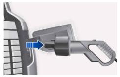
3. Press the latch on the charging connector and pull the charging connector to remove the adapter.
