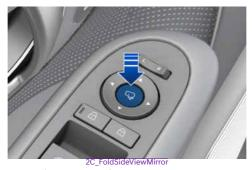
The side view mirrors can be folded or unfolded by pressing the button.
