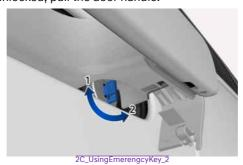
3. After using the mechanical key, turn the key knob and insert the key protector.
