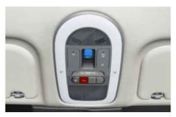
The sunroof can only be operated when the Start/Stop button is in the POWER ON or DRIVE READY position.
