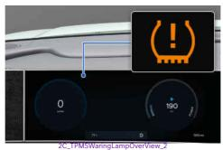
The TPMS Malfunction (!) Indicator illuminates after it blinks for about one minute when there is a problem with the Tire Pressure Monitoring System. Have the system inspected by an authorized HYUNDAI dealer as soon as possible.
