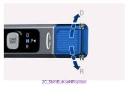
To shift the gear to N (Neutral), rotate the rotary gear shift dial to N (Neutral) while depressing the brake pedal.
