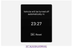
When all the conditions are satisfied, the Vehicle Auto-Shut Off operates and turns the vehicle off automatically after 60 minutes.
