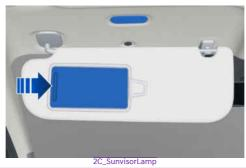
Opening the lid of the vanity mirror. The vanity mirror lamp turns on when the lid is opened and off when the lid is closed.
