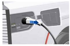
3. Press the latch on the charging connector and pull the charging connector to remove the adapter.
