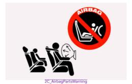
Even though your vehicle is equipped with the Occupant Classification System (OCS), never install a Child Restraint System in the front passenger's seat. An inflating airbag may forcefully strike a child or child restraint resulting in serious or fatal injury.
