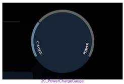
The CHARGE/POWER gauge displays the charging and discharging status of the electric energy produced by the regenerative braking and the energy consumption of the electric motor.
