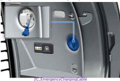
If the unlock button is not functioning properly due to a discharged battery or abnormal electrical wiring, the charging connector cannot be disconnected from the vehicle.
