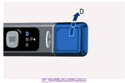
To shift the gear to D (Drive), rotate the rotary gear shift dial to D (Drive) while depressing the brake pedal.
