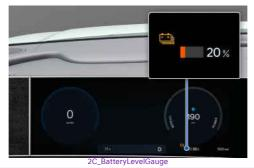
The SOC indicator is displayed at the bottom of the CHARGE/POWER gauge and shows the charge level of the high voltage battery as a percentage. The lower the number, the more the vehicle needs to be charged, and 100 % indicates a full charge.
