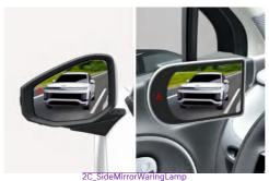
SEW warns the driver with a warning message and an audible warning. The warning light on the side view mirrors also blinks to warn you.
