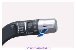
To spray washer fluid on the camera, slide the wiper switch toward the cluster.
