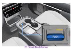
Press the DRIVE/TERRAIN button to change from normal driving mode to multi terrain mode. Press the button up or down to select SNOW, MUD, or SAND.
