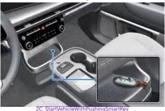
If the vehicle does not start due to a dead smart key battery or radio interference, place the smart key in the emergency start symbol position located in the center console open tray.
