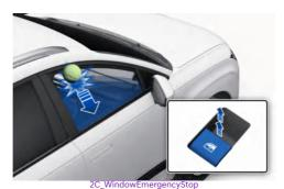
If a window senses any obstacle while it is closing automatically, it stops and lowers about 12 in. (30 cm) to allow the object to be cleared.
