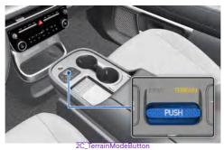
The terrain mode helps achieve optimal driving performance by controlling vehicle and braking according to the road conditions.
