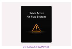
The AAF system may not operate normally if the air flap is temporarily opened due to foreign factors or if the controller is contaminated by snow or rain, etc.
