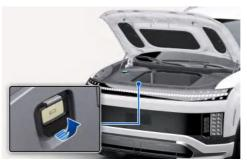
Open the button cover located inside the front trunk upwards and press the emergency front trunk release button.
