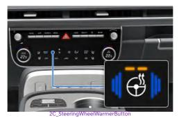
When the Start/Stop button is in the POWER ON position or when the vehicle is running, press the steering wheel heater button to warm the steering wheel.
