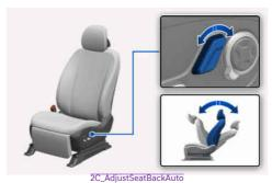
Push the control switch forward or rearward to adjust the seatback angle.
