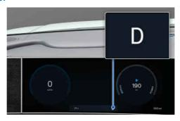
The Gear Shift Indicator indicates the current gear or P (Park).
