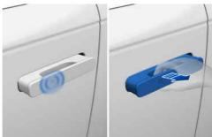
Touch the front door lock/unlock sensor (engraved part) on the driver's outside door handle.
