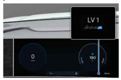
The regenerative brake indicates the level of the regenerative braking that you set. And it also indicates Smart regenerative system's operation status.
