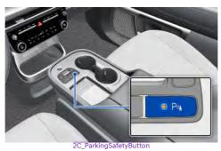
Press and hold the Parking Safety Pv button to turn the Reverse PCA on or off.
