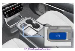
Press and hold the Parking/View [P] button to turn on RSPA. Also, Parking Distance Warning (PDW) and Surround View Monitor (SVM) automatically turns on.
