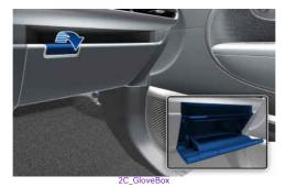
To open, pull the lever. Always close the glove box door after use.
