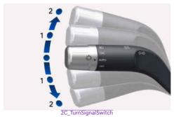
To signal a turn, completely push down (position 2) on the lever for a left turn or up (position 2) for a right turn.
