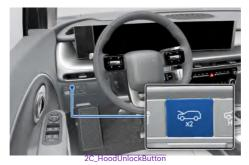
• After pressing the hood unlock button once, you must press it again within about 3 seconds to unlock the hood. If about 3 seconds have passed, it will be reset and you will have to press the hood unlock button twice again.
