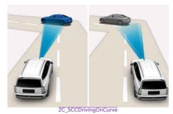
On curves, SCC may not detect a vehicle in the same lane, and may accelerate to the set speed. Also, vehicle speed may rapidly decrease when the vehicle ahead is detected suddenly.
