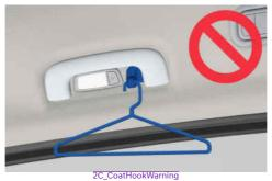
Only hang soft clothing without heavy, sharp or breakable objects in the clothes pockets. In a collision or when the curtain airbag is inflated, the objects could move and cause serious injury.
