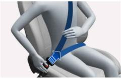
Press the release button in the locking buckle.
