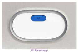
ক্ল: Press the button to turn on and off the rear lamp.
