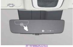
If the symbol shown in the illustration is displayed when using the Digital Center Mirror in digital mirror mode, the system may be malfunctioning. The symbol will disappear in a
