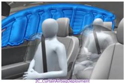
Curtain airbags are located along both sides of the roof rails above the front and rear doors.
