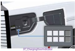
Check the State of Charge (SOC) of the high voltage battery via the charge indicator light inside the charging door with the vehicle door unlocked.
