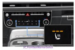
While the vehicle is running, touch the icon to warm the driver's seat or front passenger's seat.
