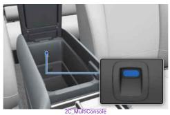
The two-way multi console lamp turns on when you turn on the interior button lights while the Start/Stop button is in the POWER ON or DRIVE READY position.
