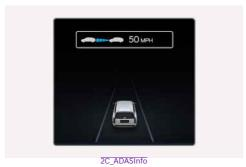
The current operation condition of Manual Speed Limit Assist, Smart Cruise Control, Lane Following Assist, etc. appears.
