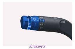
The parking lights, license plate light, and instrument panel light turn ON when you turn the knob to the 30% position.
