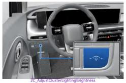
When the vehicle's parking lights or headlights are on, press the illumination control switch to adjust the brightness of the instrument panel illumination.
