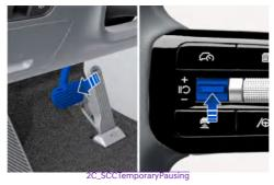
Press the II a switch or depress the brake pedal to temporarily cancel SCC.
