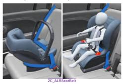
When not using the LATCH system, all Child Restraint Systems must be secured to a rear seat using the lap/shoulder belt.
