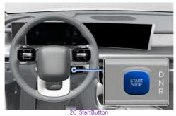
Whenever the front door is opened, the Start/Stop button illuminates and goes off for a few minutes after the door is closed.
