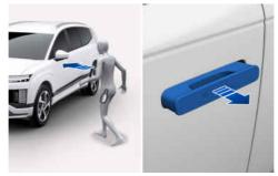
Approach within 1 m (40 in.) to the front outside door handle while carrying the smart key.
