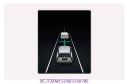
HDA operates on main roads of highway, and does not operate on interchanges or junctions.
