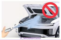
Water washing in the motor compartment including high pressure water washing may cause the failure of electrical circuits located in the motor compartment.
