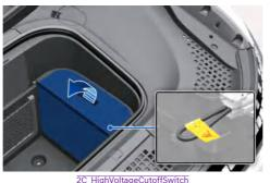
High voltage cut-off switch is a device located inside the motor compartment to block the battery's high voltage when your vehicle is inspected at an authorized HYUNDAI
