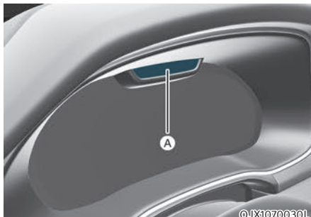
[A] : Interior view camera
