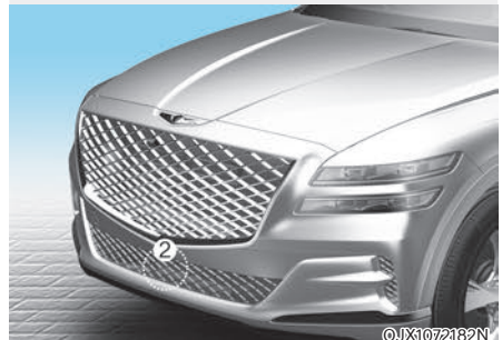
[1] : Front view camera, [2] : Front radar
