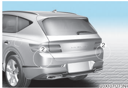
[1] : Front view camera, [2] : Rear corner radar
