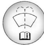
Open the cap with the washer symbol on it. Add washer fluid until the tank is full. See *Engine Compartment Overview* ⇨ 218 for reservoir location.
