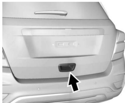
To open the liftgate, press
