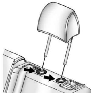
2. Press both buttons on the head restraint posts at the same time, and pull up on the head restraint.
