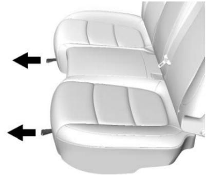
4. Pull the strap on the front edge of the rear seat cushion to release the cushion. Tilt the seat cushion forward toward the front of the vehicle.
