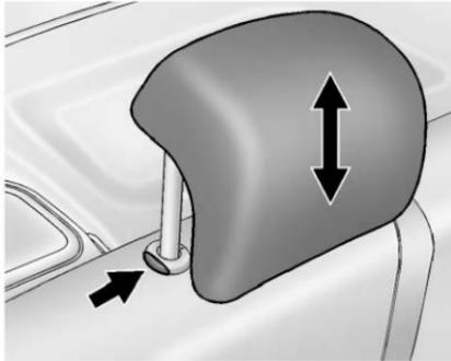
To lower the head restraint, press the button, located on the top of the seatback, and push the head restraint down.
