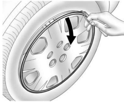
2. Remove the wheel cover, if the vehicle has one, to reach the wheel bolts.
