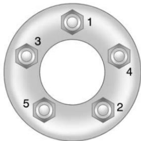
14. Tighten the wheel nuts firmly with the wheel wrench in a crisscross sequence, as shown.
