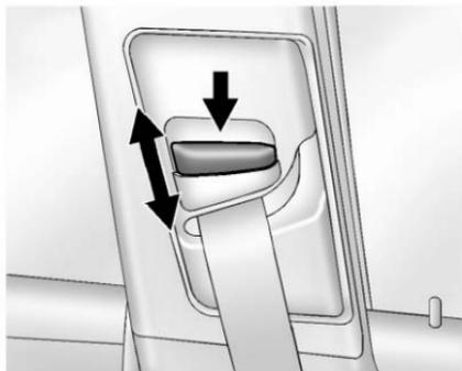
To move the shoulder belt height adjuster down, push down on the release button and move the height adjuster to the desired position. You can move the height adjuster up by pushing up on the shoulder belt guide.
