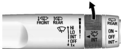
**INT** : Move the lever up to INT for intermittent wipes, then turn the
