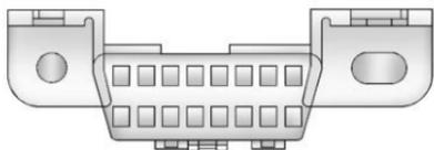
The DLC is under the instrument panel to the left of the steering wheel. Connecting devices that are not used to perform an Emissions Inspection/Maintenance test or to service the vehicle may affect vehicle operation. See *Add-On Electrical Equipment* ⇨ 212. See your dealer if assistance is needed.
