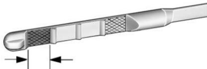
If the oil is below the cross-hatched area at the tip of the dipstick and the engine has been off for at least
