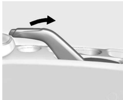
With the brake pedal applied, pull up firmly on the parking brake handle without pressing the release button. See *Shifting Into Park* ⇨ 182 or *Parking (Manual Transmission)* ⇨ 184. If the ignition is on, the brake system warning light will come on. See *Brake System Warning Light* ⇨ 105.
