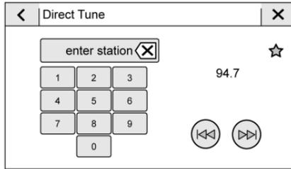
Access Direct Tune by touching the Tune icon on the AM, FM, or SXM screen to bring up the keypad. Navigate up and down through all frequencies using **⏪** or **⏩**. Directly enter a station or channel using the keypad. When a new station or channel is entered, the information about that station or channel displays on the right side. This information will update with each new valid frequency tuned to.
