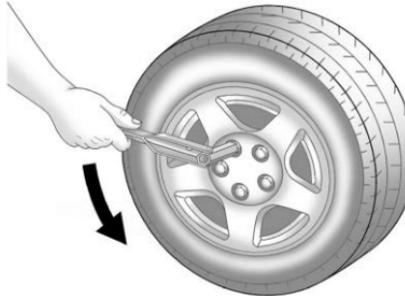
3. Turn the wheel wrench counterclockwise to loosen the wheel nuts. Do not remove them yet.
