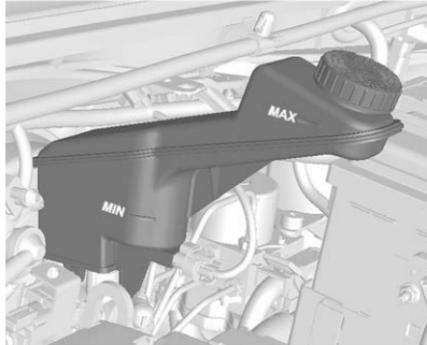
With the vehicle in P (Park) on a level surface, the brake fluid level should be between the minimum and maximum marks on the brake fluid reservoir.
