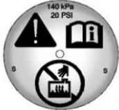
1. Remove the coolant surge tank pressure cap when the cooling system, including the coolant surge tank pressure cap and upper radiator hose, is no longer hot.
