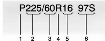
**(1) Passenger (P-Metric) Tire :** The United States version of a metric tire sizing system. The letter "P" as the first character in the tire size means a passenger vehicle tire engineered to standards set by the U.S. Tire and Rim Association.
