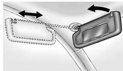
Pull the sun visor down to block glare. If equipped, detach the sun visor from the center mount to pivot to the side window or to extend along the rod.
