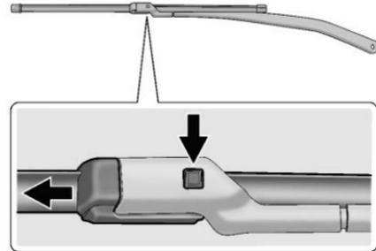
2. Press the release button on the top side of the wiper and pull the wiper blade out of the end of the wiper arm.
