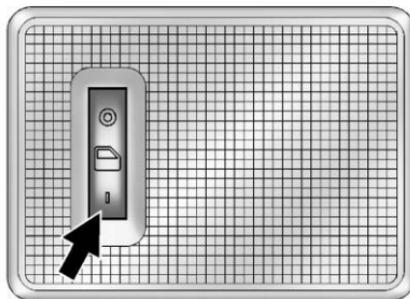
The rear dome lamp controls are in the headliner above the rear seats.
