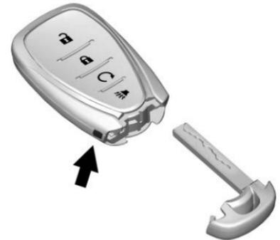
1. Press the button on the side of the RKE transmitter and pull the key out. Never pull the key out without pressing the button.
