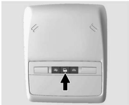
The front dome lamp controls are in the overhead console.
