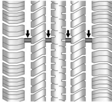
Treadwear indicators are one way to tell when it is time for new tires. Treadwear indicators appear when the tires have only 1.6 mm (1/16 in) or less of tread remaining. See *Tire Inspection* ⇨ 267 and *Tire Rotation* ⇨ 268.
