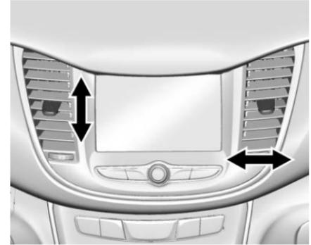
Use the air vents in the center and on the side of the instrument panel to direct the airflow. Move the slats on the center air vents to direct airflow.
