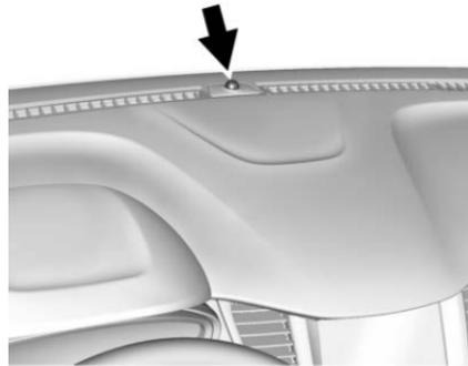
An indicator light, on the instrument panel near the windshield, indicates the status of the system:
