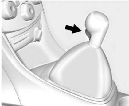
**R (Reverse)** : To engage R (Reverse), with the vehicle stationary, pull up on the button on the shift lever and engage the gear. If the gear does not engage, set the lever in Neutral, release the clutch pedal, and apply it again; then repeat gear selection.
