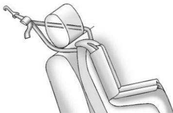
If the position you are using has an adjustable headrest or head restraint and you are using a dual tether, raise the headrest or head restraint and route the tether under the headrest or head restraint and around the headrest or head restraint posts.
