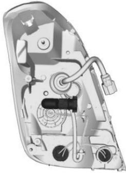
4. Remove the old bulb from the bulb socket by pulling it straight out.
