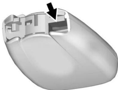
2. Separate the two halves of the transmitter using a flat tool inserted into the area near the key slot.
