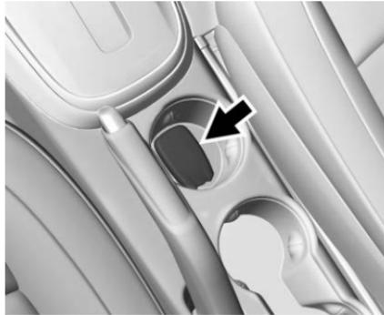
1. Place the transmitter in the front cupholder of the center console storage area.
