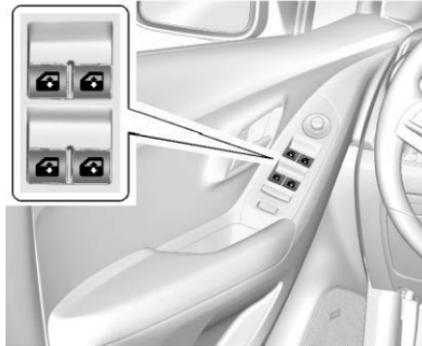
Power windows work when the ignition is on, in ACC/ACCESSORY, or when Retained Accessory Power (RAP) is active. See *Retained Accessory Power (RAP)* ⇨ 181.
