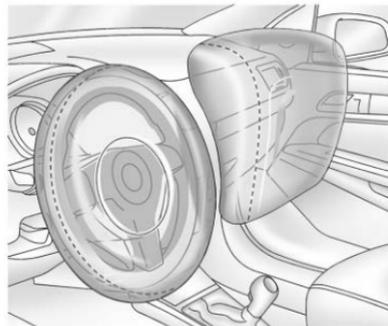
The driver frontal airbag is in the center of the steering wheel.
