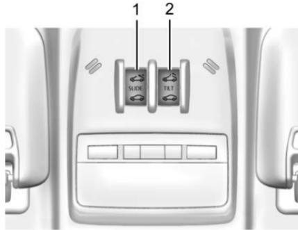
If equipped, the sunroof only operates when the ignition is on or when Retained Accessory Power (RAP) is active. See *Retained Accessory Power (RAP)* ⇨ 181.
