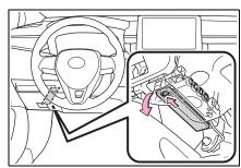
Remove the fuse with the pullout tool.
