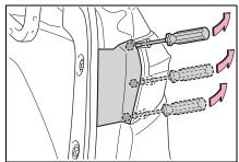
3 Pull the cover toward the rear of the vehicle and remove the cover.
