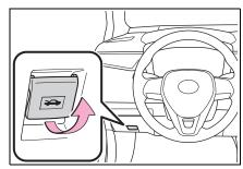
Pull the auxiliary catch lever to the left and lift the hood.
