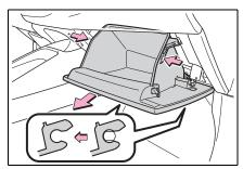
4 Unlock the filter cover (A), pull the filter cover out of the 7
