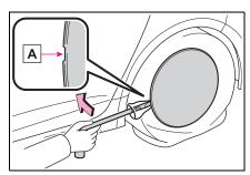
Slightly loosen the wheel nuts (one turn).
