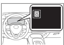
If signs other than speed limit signs are recognized, they will be displayed in an overlapping stack
