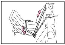
5 After installing the child restraint system, rock it back and forth to ensure that it is installed securely. (→P.63)
