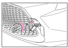
4 Tighten down the towing eyelet securely using a wheel nut wrench (if equipped) or hard metal bar.
