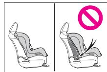
\*3: If the head restraint interferes with your child restraint system, and the head restraint can be removed, remove the head restraint.
