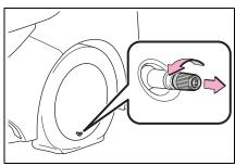
3 Extend the hose. Remove the air release cap from the hose.
