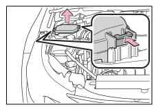
Engine compartment: type B fuse box
