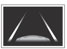
Indicates that the system is recognizing white (yellow) lines or a course\*. When the vehicle departs from its lane, the white line displayed on the side the vehicle departs from flashes orange.
