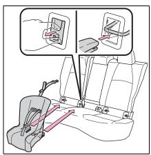
If the child restraint has a top strap, follow the child restraint manufacturer's operation manual regarding the installation, using the top strap to latch onto the top strap anchorage. (→P.68)
