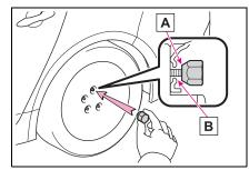
When replacing an aluminum wheel with a steel wheel (including a compact spare tire), tighten the wheel nuts until the tapered portion A comes into loose contact with the disc wheel seat B.
