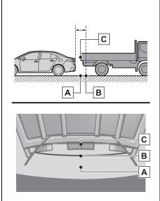
Visually check the surroundings and the area behind the vehicle. On the screen, it appears that a truck is parking at point B. However, in reality if you back up to point A, you will hit the truck. On the screen, it appears that A is closest and C is farthest away. However, in reality, the distance to A and C is the same, and B is farther than A and C.
