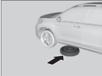
8. Place the compact spare tire (wheel side up) under the vehicle body, near the tire that needs to be replaced.
