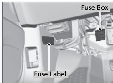
Fuse locations are shown on the image. Locate the fuse in question by the fuse number and label number.
