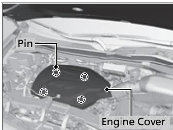
3. Pull up on the engine cover, remove it from the pins.
