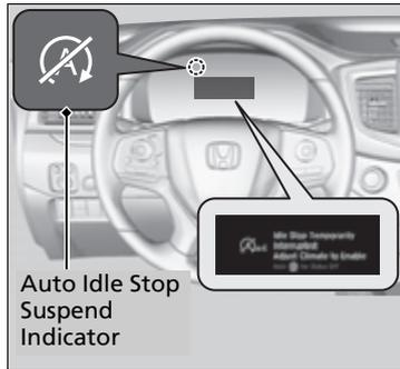
The Auto Idle Stop suspend indicator comes on and a message appears on the gauge when the Auto Idle Stop system cannot be activated.
