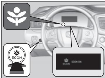
The **ECON** button turns the ECON mode on and off. The ECON mode helps you improve your fuel economy by adjusting the performance of the engine, air conditioning system, and cruise control.
