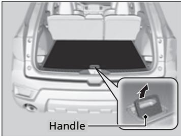
1. Push the rear edge of the handle on the cargo floor lid and open the lid.
