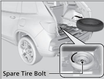
**5.** Unscrew the spare tire bolt and slide the tire to the rear of the vehicle. Remove the spare tire from vehicle.
