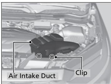
2. Remove the holding clips and the air intake duct.
