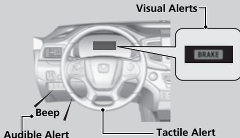
You can change the distance (**Long/Normal/Short**) between vehicles at which the system's earliest collision alert will come on through audio/information screen setting options.
