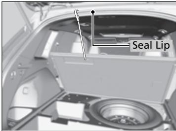
3. Attach the hook onto the weather seal lip.
