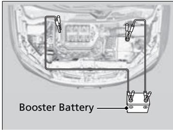
5. Connect the other end of the first jumper cable to the booster battery  $\oplus$  terminal.
