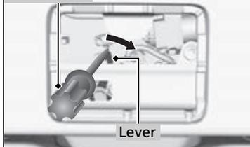
2. To open the tailgate, push the tailgate while pushing the lever to the right using a flat-tip screw driver.
