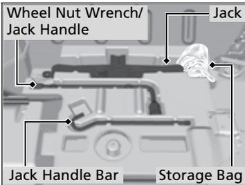
**6.** Pull out the wheel nut wrench, jack handle bar, storage bag, and jack from the tool case.
