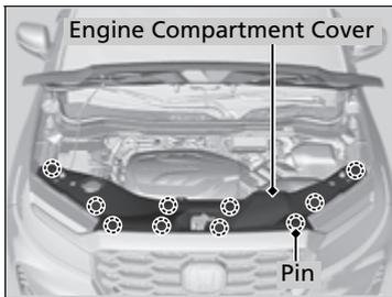
1. Pull up on the engine compartment cover, remove it from the pin holders.
