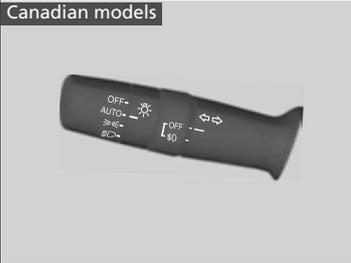
The headlights come on when you unlock a door in dark areas with the headlight switch in **AUTO**.
