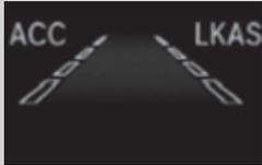
When the LKAS is suspended, the lane lines on the driver information interface change to lane outlines, and the beeper sounds (if activated).
