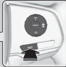
■ Press the **MAIN** button on the steering wheel.
