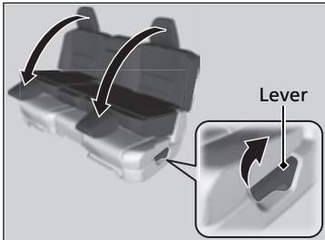
To return the seat to the original position, pull up the seat-back in the upright position.
