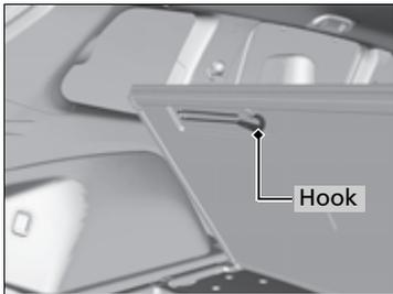
2. Lift the secondary lid, then remove the hook from the bottom of the lid.
