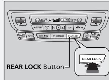
Press the **REAR LOCK** button to turn the rear lock mode on and off. While the rear lock mode is on, the rear control panel is disabled.
