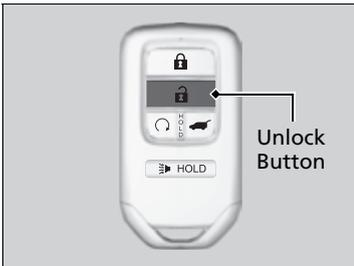
**To open:** Press the unlock button, and then within 10 seconds, press it again and hold it.
