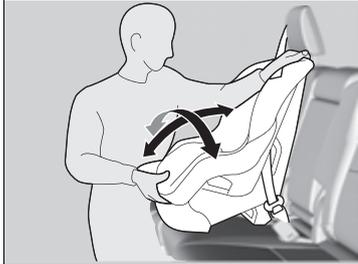
**9.** Grab the shoulder part of the seat belt near the buckle, and pull up to remove any slack from the lap part of the belt.
