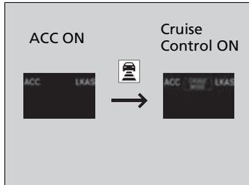
Press and hold the
