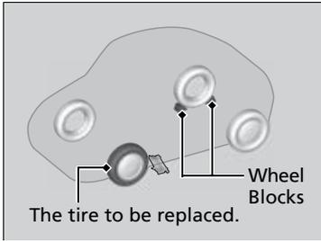
7. Place a wheel block or rock in front and rear of the wheel diagonal to the flat tire.
