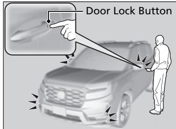
Press the door lock button on a front door or the tailgate.
