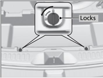
**4.** Unlock the cargo bin by turning the two locks. Remove the cargo bin from the vehicle.
