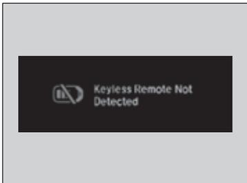
When the power mode is set to any mode other than OFF (LOCK) and you remove the keyless remote from the vehicle and shut the door, an alarm will sound. If the alarm continues to sound, place the keyless remote in another location.
