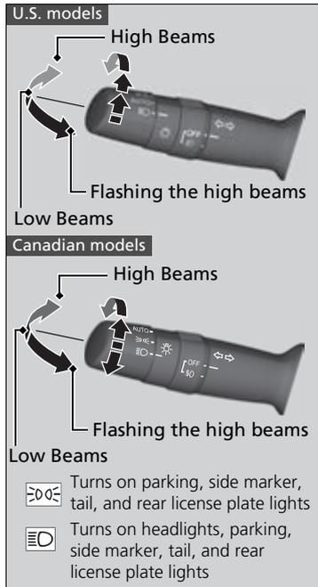
Rotating the light switch turns the lights on and off, regardless of the power mode setting.
