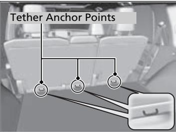
A tether anchor point is provided behind each rear seating position. If you have a child seat that comes with a tether but can be installed with a seat belt, the tether may be used for additional security.
