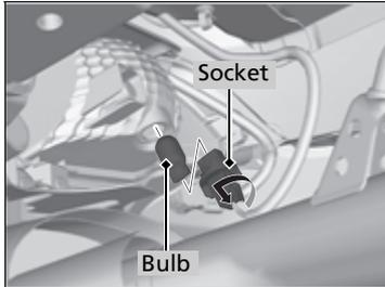
1. Turn the socket counter-clockwise and remove it. Remove the old bulb.
