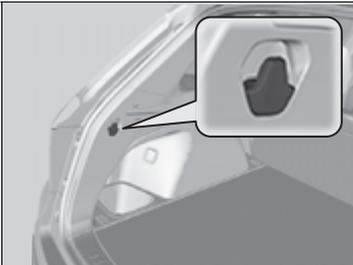
The cargo hooks on both sides of the cargo area can be used to hang a light items.
