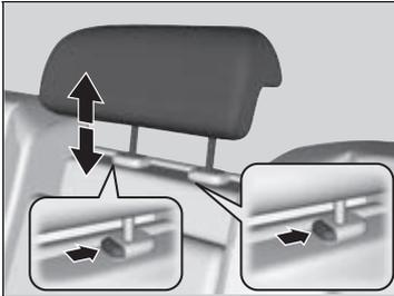
A passenger sitting in the rear center seating position should adjust the height of their head restraint to an appropriate position before the vehicle begins moving.
