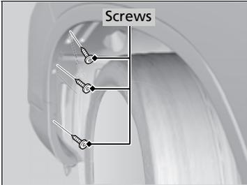
1. Remove the screws, pull the inner fender back.
