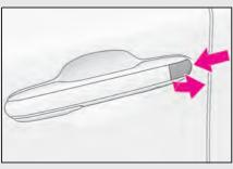
2 Remove the cover by pressing it on the rear.
