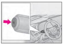
Press the Automatic High Beam switch.
