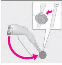
5 Remove the AC charging connector cap and secure it to the cable.
