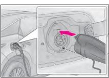
6 Insert the charging connector into the AC charging inlet.
