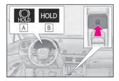
Turns the brake hold system on
