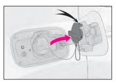
4 Remove the AC charging inlet cap and secure it into the holder on the charging port lid.
