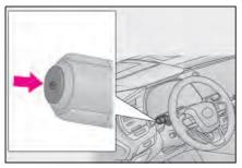
**1** Press the Automatic High Beam switch.
