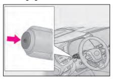
Press the Adaptive High-beam System switch.
