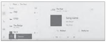
[Ch]: Touch [-] or [+] to search for the receivable channels. Touch and hold to jump to the next frequency with available radio signal. When released, the current channel is received.
