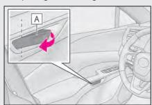
Pull the manual release handle **A** twice to open the door.
