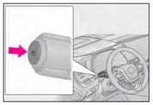
1 Press the Adaptive High-beam System switch.
