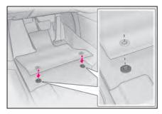
1 Insert the retaining hooks (clips) into the floor mat eyelets.
