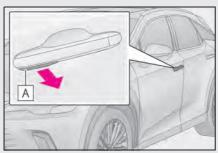
Pull the manual release handle **A** to open the door.
