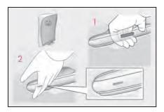
1 Grip the driver's door handle to unlock the door. Grip any passenger door handle to unlock all the doors.\*
