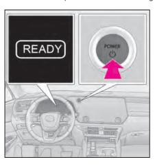
4 Press the power switch shortly and firmly.
