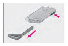
To take out the mechanical key, push the release button and take the key out.
