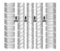
Treadwear indicators are one way to tell when it is time for new tires. Treadwear indicators appear when the tires have only 1.6 mm (1/16 in) or less of tread remaining. See *Tire Inspection* ⇒ 295 and *Tire Rotation* ⇒ 295.
