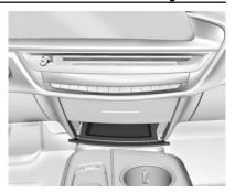
If equipped, there is an upper sliding drawer and a lower storage bin in the center of the instrument panel.
