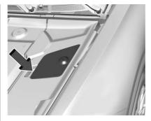
Remove the cover to access the emergency manual charge cord release handle.
