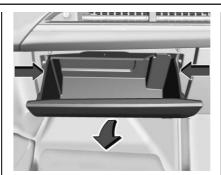
Press the sides of the glove box bin inward to clear the stoppers and turn downward to lower the bin.
