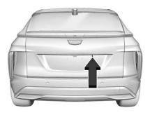
To access the liftgate key lock cylinder, insert the mechanical key into the cylinder and turn to unlock. See  $Keys \Leftrightarrow 6$ .
