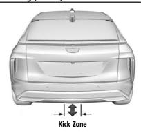
To operate, move your foot in a forward kicking motion under the left side of the rear bumper, at the location of the projected logo, then pull it back. Then step back. The kick must come within 14 cm (6 in) of the rear bumper to activate.
