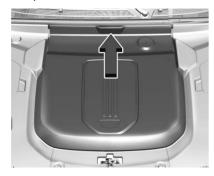
To open the lid, pull the handle to disengage the clips and remove the cover.
