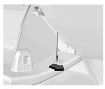
3. Unhook the string dampener to fully remove the glove box bin.
