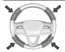
Also, the Super Cruise indicator light will turn red and a message will display in the DIC, beeps will sound, or the Safety Alert Seat will vibrate. To view available settings from the infotainment screen, touch Settings > Vehicle > Collision/Detection Systems. After you begin steering manually, then Super Cruise will disengage.
