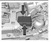
To open the fuse block cover, press the clips at the side and back and pull the cover up.
