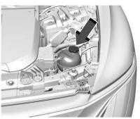
After the system has completely cooled, check that the coolant level in the reservoir.
