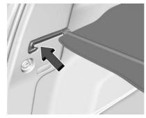
5. Insert the cargo cover pins into the channels on both sides.
