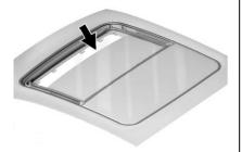
Dirt and debris may collect on the sunroof seal or in the track. This could cause an issue with sunroof operation or noise. It could also plug the water drainage system.
