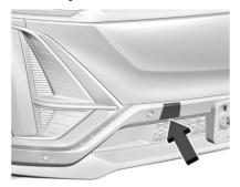
Carefully open the cover in the fascia by using the small notch that conceals the tow eye socket.
