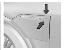
Push the top right corner of the charge port door and release to open the door.In cold weather conditions, ice may form around the charge port door. Remove ice from the area before attempting to open or close the charge port door.
