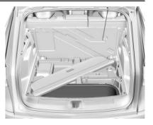
Press the handle and pull up the load floor to access.
