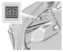
If equipped, the rear seatbacks can also be folded forward by pressing and holding the switches located in the rear cargo area.
