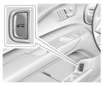
To open or close the liftgate from the inside, press  $< \sim$  .
