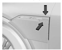
Push the rearward edge of the charge port door and release to open the door. In cold weather conditions, ice may form around the charge port door. The charge port door may not open on the first attempt. Remove ice from the area and repeat attempting to open the charge port door.
