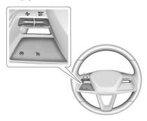
(\*\*): Press to turn the system on or off. A white indicator comes on in the instrument cluster when cruise control is turned on.
