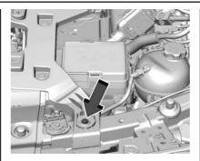
3. Remove the bolt to access the fuse block.
