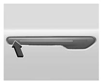
All outside door handles will deploy whenever the doors are unlocked, or when any door is opened or closed. The handles can also be programmed to deploy when the remote key approaches. To view available settings from the infotainment screen, touch Settings > Vehicle > Remote Lock, Unlock, Start.
