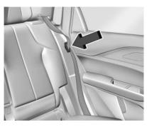
Stow the seat belt latch plate in the stowage slot.
