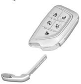
To remove the mechanical key, press the button near the bottom of the remote key, and pull the key out. Never pull the mechanical key out without pressing the button.
