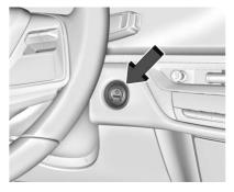
The vehicle has an electronic pushbutton start.
