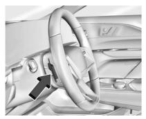
Applying the Regen on Demand steering wheel paddle requests additional deceleration using regenerative braking. The deceleration request increases as the paddle is applied more. It works in D (Drive). The accelerator pedal can be used to manage deceleration while using Regen on Demand. See One-Pedal Driving \$\Display\$ 180.
