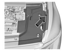
The Underhood Compartment Fuse Block is under a cover and side extension/ shield in the underhood compartment. Unclip right side of shield and remove the right side access cover.
