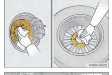
2 Install the spare tire and loosely tighten each nut by hand to approximately the same amount.
