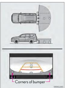
The parking assist monitor displays an image of the view from the bumper of the rear area of the vehicle.
