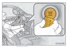
3 Firmly depress the brake pedal and check that information display.
