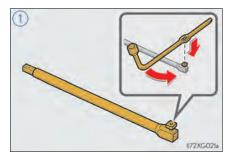
② Assemble the jack handle extension bar and wheel nut wrench and tighten the bolt.
