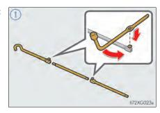
2 Assemble the jack handle bar, jack handle extension bar and wheel nut wrench and tighten the bolts.
