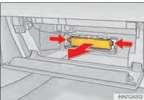
4 Slide and pull out the filter. Replace the filter with a new one.
