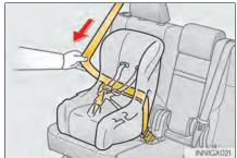
Shill be pushing the child restraint system into the seat, allow the shoulder belt to retract until the child restraint system is securely in place.
