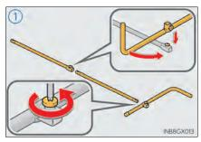
Assemble the jack handle extension bar and the jack handle and tighten the bolt and the screw.
