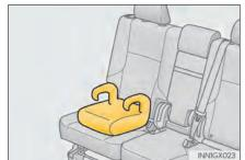
3 Sit the child in the child restraint system. Fit the seat belt to the child restraint system according to the manufacturer's instructions and insert the plate into the buckle. Make sure that the belt is not twisted.
