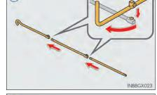
3 Assemble the jack handle extension bar and the jack handle and tighten the screw.
