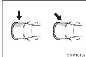
The SRS side airbags do not generally inflate if the vehicle is involved in a frontal or rear collision, if it rolls over, or if it is involved in a low-speed side collision.
