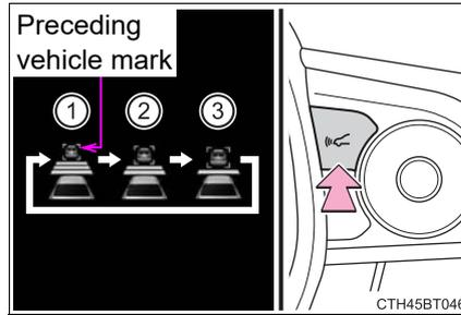
**Vehicle-to-vehicle distance settings (vehicle-to-vehicle distance control mode)**
