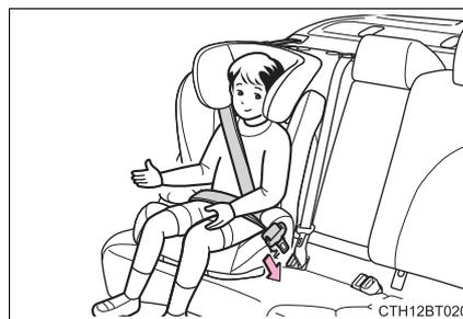
Check that the shoulder belt is correctly positioned over the child's shoulder and that the lap belt is as low as possible. (→P. 28)
