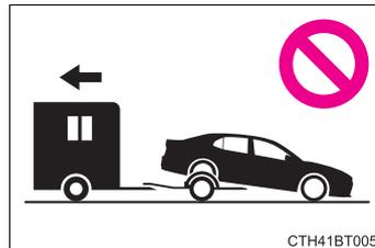
■ **To prevent causing serious damage to the transmission and AWD system (AWD models)**
