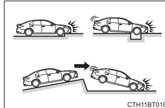
The SRS curtain shield airbags may also deploy under the situations shown in the illustration.
