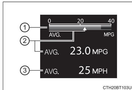
Displays the average vehicle speed since reset or elapsed time since reset, as selected in . (→P. 100)
