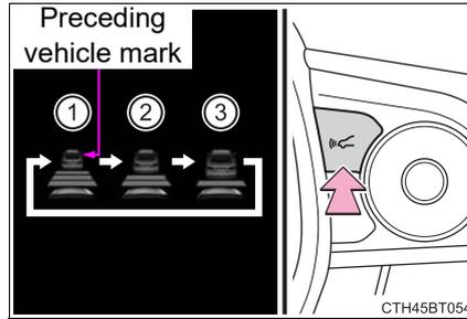
**Vehicle-to-vehicle distance settings (vehicle-to-vehicle distance control mode)**
