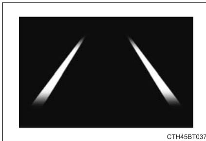
Indicates that the system is recognizing white (yellow) lines. When the vehicle departs from its lane, the white line displayed on the side the vehicle departs from flashes yellow.
