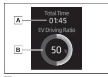
A Elapsed time after starting Displays the elapsed time since hybrid system was started.<sup>\*</sup>
