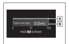
A Current fuel consumption Displays instantaneous current fuel consumption.
