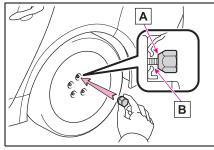
When replacing an aluminum wheel with a steel wheel (including a compact spare tire), tighten the wheel nuts until the tapered portion  $\boxed{A}$  comes into loose contact with the
