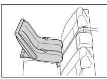
2 Run the seat belt through the child restraint system and insert the plate into the buckle. Make sure that the belt is not twisted.
