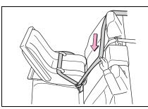
4 While pushing the child restraint system down into the rear seat, allow the shoulder belt to retract until the child restraint system is securely in place.
