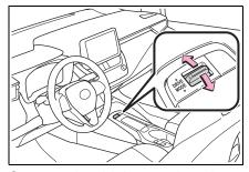
Operate the driving mode select switch forward or backward to select the desired driving mode on the multi-information display.
