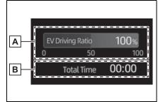
A EV driving ratio after starting Displays the percentage of EV driving since the hybrid system was started.<sup>\*</sup>
