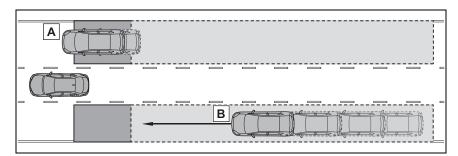
A Vehicles that are traveling in areas that are not visible using the outside rear view mirrors (the blind spots)
