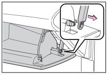
3 Push in the glove box on the vehicle's outer side to disconnect the claws. Then pull out the glove box and disconnect the lower claws.
