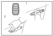
1 Grip the driver's door handle to unlock the door. Holding the driver's door handle for approximately 2 seconds unlocks all the doors. Grip the front passenger's door handle to unlock all the doors.\*
