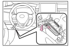
Remove the fuse with the pullout tool.
