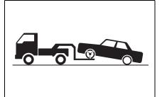
Release the parking brake. Turn automatic mode off.  $(\rightarrow P.184)$
