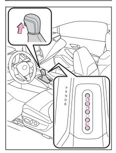
While the power switch is in ON and the brake pedal depressed<sup>\*</sup>, shift the shift lever while pushing the shift release button on the shift knob.
