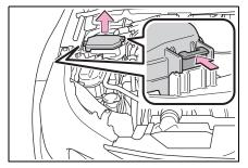
Engine compartment: type B fuse box
