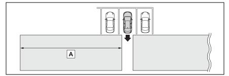
The buzzer can alert the driver of faster vehicles approaching from farther away.
