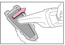
**5** Hold the filter to the light and check if it is not clogged.
