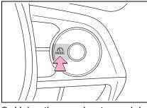
2 Using the accelerator pedal, accelerate to the desired vehicle speed (approximately 20 mph [30 km/h] or more), and press the driving assist switch to set the set vehicle speed.
