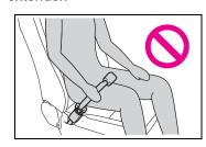
The SRS front passenger airbag also deploys with considerable force, and can cause death or serious injury especially if the front passenger is very close to the airbag. The front passenger seat should be as far from the airbag as possible with the seatback adjusted, so the front passenger sits upright. 1
