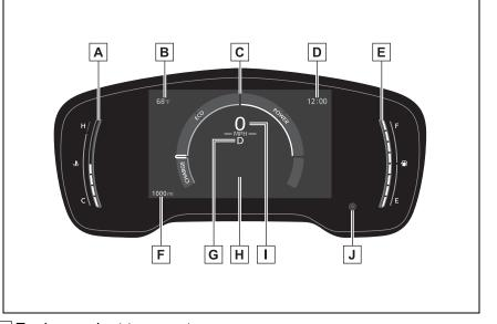
A Engine coolant temperature gauge
