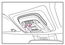
1 Turns the door position on/off When a door is opened while the door position is on, the lights turn on.
