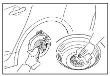
2 Install the tire and loosely tighten each wheel nut by hand by approximately the same amount.
