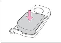
6 Operate the **a** or **a** switch and check that the doors can be locked/unlocked.
