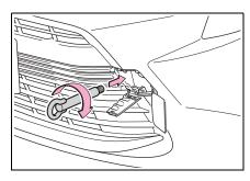
4 Tighten down the towing eyelet securely using a wheel nut wrench (if equipped) or hard metal bar.
