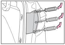
3 Pull the cover toward the rear of the vehicle and remove the cover.
