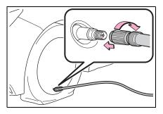
8 Remove the power plug from the compressor.
