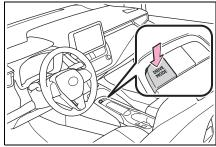
Each time the switch is pressed, the system changes between Eco drive mode and normal mode.
