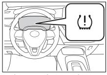
9 If the specified tire inflation pressure of the wheel set installed differs from that of the previous set, it will be necessary to perform the tire inflation pressure setting procedure of the tire pressure warning system. (→P.333)
