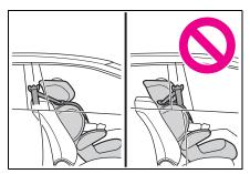
When installing a junior seat, if the child in your child restraint system is in a very upright position, adjust the seatback angle to the most comfortable position. And if the seat belt shoulder anchor is ahead of the child seat belt guide, move the seat cushion forward.
