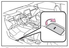
Trunk release button (vehicles with a smart key system)
