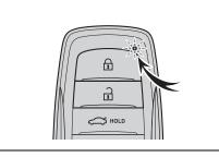
Electronic keys that will not be used for long periods of time can be set to the battery-saving mode in advance.
