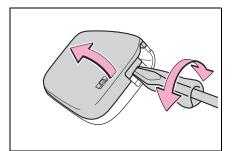
3 Remove the depleted battery using a small flathead screwdriver.
