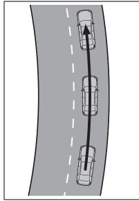
When the function is operating, if the vehicle is likely to depart from its lane, the driver will be alerted via a display and buzzer.
