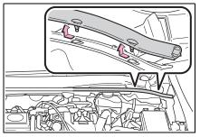
2 Disconnect the claws and remove the service cover.
