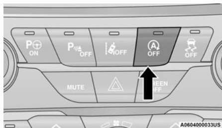
Stop/Start OFF Switch
