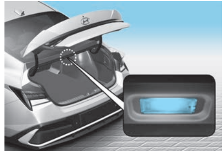
Trunk room lamp
