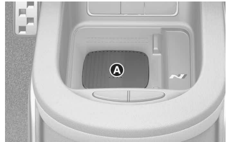
[A] Vehicle authentication pad (wireless charging pad)
