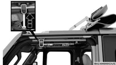
Attach Front Door Rail Bolt
