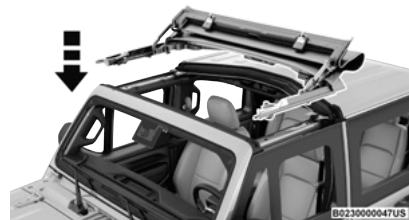
Lower Sunrider® Onto The Vehicle
