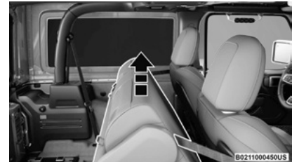
Rear Seat Tumble Position Retention Strap
