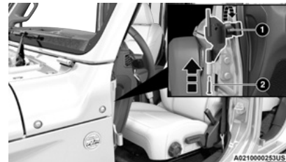
Attaching Mirror Bracket To The Vehicle
