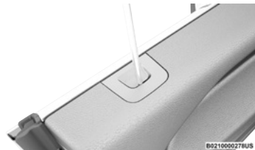
Place Tool Into Service Hole Of Plug To Remove
