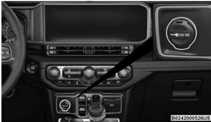
Front Power Outlet
