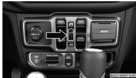
Window Lockout Switch
