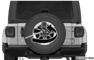
Removing The Spare Tire
