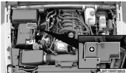
Positive (+) Battery Post
