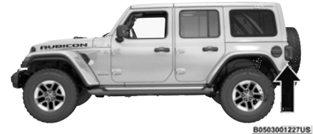
BSM Radar Location (Left Side Shown)
