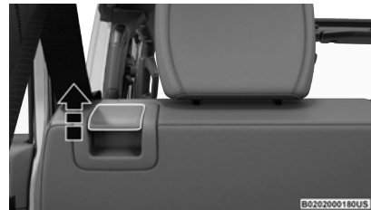
Lift Seatback Release Lever Up
