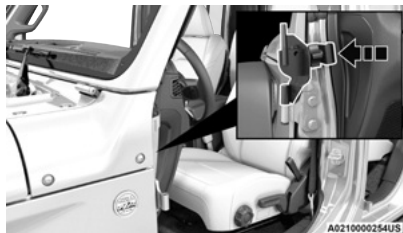
Push Bracket Onto A-pillar
