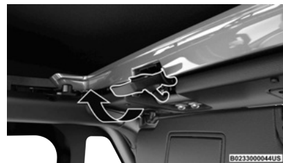
Engage Both Header Latches
