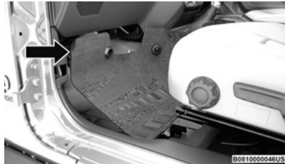
Front Carpet Pulled Away
