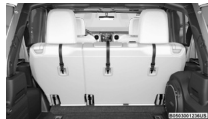
Tether Strap Mounting (Four-Door Models Without Center Armrest)
