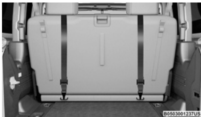
Tether Strap Mounting (Two-Door Models)
