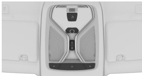
Opening/closing the glass sunroof/sun protection.
