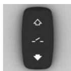
Opening/closing the glass sunroof/sun protection.
