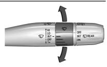
**INT :** If equipped with intermittent wipers only, move the windshield wiper lever to INT. Turn the band up for more frequent wipes or down for less frequent wipes.
