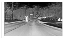
With the Pedestrian Braking system turned on, Night Vision provides a red Head-Up Display (HUD) alert when the system detects that the vehicle is approaching a pedestrian ahead too quickly. In addition, an alert beeps or the Safety Alert Seat pulses, if equipped. See *Front Pedestrian Braking (FPB) System*  $\Rightarrow$  323.
