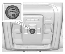
The power liftgate switch is on the overhead console. The vehicle must be in P (Park).
