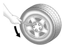
3. Use the wheel wrench to loosen all the wheel nuts. Turn the wheel wrench counterclockwise to loosen the wheel nuts. Do not remove the wheel nuts yet.
