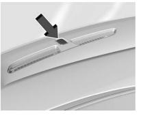
The vehicle has a light sensor on the top of the instrument panel that controls the automatic headlamp
