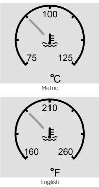
This gauge displays on the infotainment display. If show in cluster is selected a digital value is shown on the instrument cluster in the left zone.
