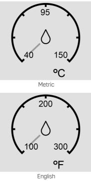
The transmission temperature gauge shows the transmission fluid temperature. If the gauge is reading in the red area and/or a message appears in the Driver Information Center (DIC), the vehicle must be stopped and the cause checked. One possible cause is a low fluid level in the transmission.
