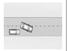
Super Cruise may not detect a vehicle that enters your lane, or may not brake fast enough to avoid a crash. You must manually brake and steer the vehicle.
