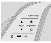
The HUD control is on a touchscreen to the left of the instrument cluster. HUD controls are also available on the infotainment screen. See *Settings*  $\Rightarrow$  205.
