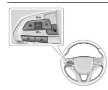
$\mathfrak{G}$ : Press to turn the system on or off. The indicator turns white on the instrument cluster when ACC is turned on.
