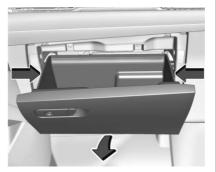
2. Press the sides of the glove box bin inward to clear the stoppers and rotate downward to lower the bin.
