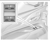
Power windows work when the ignition is on, in ACC/ACCESSORY, or when Retained Accessory Power (RAP) is active. See *Retained Accessory Power* (*RAP*)  $\Rightarrow$  250.
