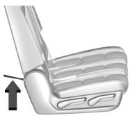
2. Pull the strap on the bottom rear of the second row seat to release the seatback. The seatback will fold forward.
