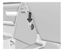
3. Unhook the string dampener to fully remove the glove box bin.
