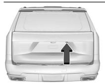
Press the button above the license plate to open the liftglass, or press  $\frac{2}{\sqrt{2}}$  twice quickly on the remote key. Do not leave the liftglass open when raising the liftgate.
