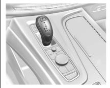
The shift pattern is displayed in the top of the shift lever. The selected gear position will illuminate red on the shift lever, while all others will be displayed in white. If the shift is not immediate, as in very cold conditions, the indicator on the shift lever may flash until it is fully engaged.
