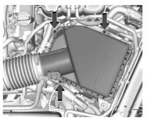
1. Remove the three screws, tilt the cover, and slide it out of the assembly.
