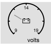
When the ignition is on, the voltmeter gauge indicates the battery voltage.
