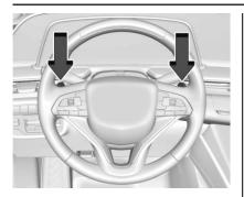
Electronic Range Select (ERS), or Manual Mode, allows manual selection of gear positions. Use this mode when driving downhill or towing a trailer to limit the top gear and vehicle speed. The shift position indicator within the Driver Information Center (DIC) displays a number next to the L indicating the highest available gear.
