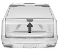
• Press the emblem under the liftglass, after unlocking all doors. A locked vehicle can be opened if the remote key is within 1 m (3 ft) of the emblem.
