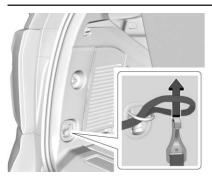
4. Remove the flat tire secure strap from the glove box and place the loop end of the strap through the cargo tie-down. Place the hook end of the strap through the loop and pull it until the strap is fastened securely to the tie-down.
