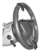
To adjust the power tilt and telescoping steering wheel:
