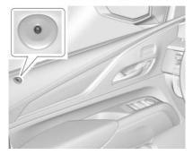
The indicator light, on the driver door near the window, indicates the status of the system. See *Power Door Locks* ⇔ *17*
