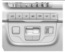
To activate each mode, press the MODE button on the instrument panel to the left of the steering wheel. To activate Terrain Mode, press button located next to the MODE button.
