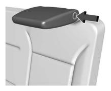
The head restraint will fold forward automatically.
