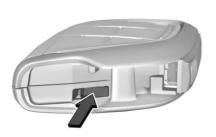
2. With the mechanical key removed, insert a flat, thin object in the center of the remote key to separate and remove the back cover.
