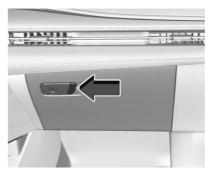
To open, pull the handle to the left. To close, push the glove box up until it latches. Use the vehicle key to lock or unlock.
