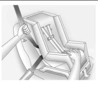
5. To tighten the belt, push down on the child restraint, pull the shoulder portion of the belt to tighten the lap portion of the belt, and feed the shoulder belt back into the retractor. When installing a forward-facing child restraint, it may be helpful to use your knee to push down on the child restraint as you tighten the belt.
