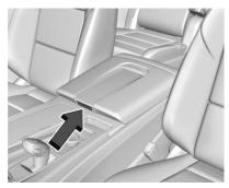
Press the button and lift to open. There is an auxiliary jack, USB ports, an accessory power outlet, a tote compartment, and a device holder inside.
