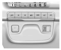
If equipped, the transfer case controls are used to shift into and out of four-wheel drive. To shift the transfer case, press the desired button. The graphic in the instrument cluster will flash while a shift is in progress. The graphic displayed will change to indicate the setting requested.
