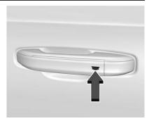
The remote key must be within 1 m (3 ft) of the liftgate or door being opened or locked. To unlock and open any door, press the touchpad on the inside grip area of the outside door handle. Touch the sensor on the front outside door handle to lock. See "Keyless Access Operation" in *Remote Keyless Entry (RKE) System Operation*  $\Rightarrow$  7.
