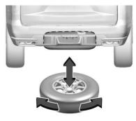
7. Make sure the tire is stored securely. Push, pull, and then try to turn the tire. If the tire moves, use the wheel wrench to tighten the cable.
