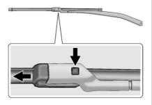
2. Press the button in the middle of the wiper arm connector, and pull the wiper blade away from the arm connector.
