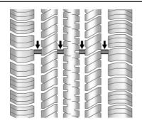
Treadwear indicators are one way to tell when it is time for new tires. Treadwear indicators appear when the tires have only 1.6 mm (1/16 in) or less of tread remaining. See *Tire Inspection*  $\Rightarrow$  *416* and *Tire Rotation*  $\Rightarrow$  *417* for additional information.
