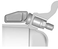
Contact your trailer service center or tire service center to have the pressure sensors installed inside the trailer tires. The technician should insert the sensor stem through the hole in the trailer wheel. When the sensor is correctly positioned, the nut on the sensor stem should be tightened to  $8 N \cdot m$  (6 lb ft). When mounting the trailer tire onto the trailer wheel be careful not to damage the sensor.
