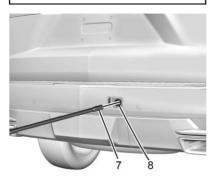
4. Insert the open end of the extension (7) through the hole in the rear bumper (8) (hoist shaft access hole).
