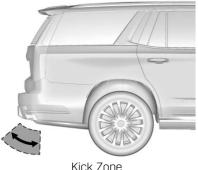
To operate, move your foot in a forward kicking motion near the center of the rear bumper at the location of the projected logo, then pull it back. The kick must come within 14 cm (6 in) of the rear bumper to activate. Then step back.
