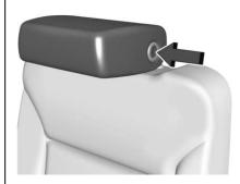
The head restraint will fold forward automatically.
