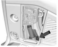
Turn the jack knob counterclockwise to release the jack and wheel blocks from the bracket. If equipped, remove the wheel blocks from the jack and place the wheel blocks on both sides of the tire at the opposite corner of the tire being changed. See *If a Tire Goes Flat* \$\\$423 for more information on the placement of the wheel blocks. Place the jack and wheel blocks near the tire being changed.
