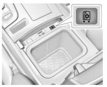
If equipped with a center console refrigerator/freezer, lift the armrest to access. A light will turn on when the armrest is up.
