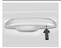
2. Insert the mechanical key into the slot at the bottom of the handle and push upward all the way until the cover frees. Do not pry or pull on the key.
