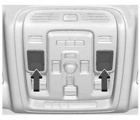
There are reading lamps in the overhead console and the headliner, if equipped.
