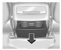
If equipped with cupholders in the back center console, press the cover and release to access. There may be two USB ports, two HDMI ports, and a power outlet on the back of the center console.
