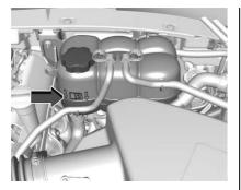
Check to see if coolant is visible in the coolant surge tank. If the coolant inside the coolant surge tank is boiling, wait until it cools down. The coolant level should be at or above the indicated mark. If it is not, there may be a leak in the cooling system.
