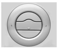
Press on the center vane rear edge to open the round outlet. Use the center vane to rotate the outlet and change the direction of the airflow. Press on the center vane leading edge to shut off the air flow.
