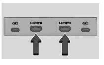
The HDMI input allows an HDMI A/V cable to be connected from an auxiliary device such as a camcorder, video game system, or Apple device. A cable from Apple is required for Apple devices.
