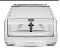
To open the liftgate, press a on the power door lock switch or press a on the remote key twice to unlock all doors, then press the emblem. Once opened, raise the liftgate using the handle on the interior bottom edge.
