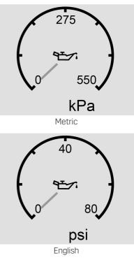
The engine oil pressure gauge shows the engine oil pressure in kPa (kilopascals) or psi (pounds per square inch) when the engine is running.
