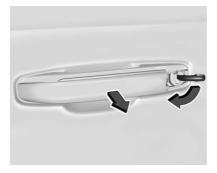
4. Insert the mechanical key in the cylinder.
