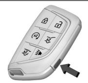
To remove the mechanical key, press the button near the bottom of the remote key, and pull the mechanical key out. Never pull the mechanical key out without pressing the button.
