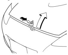
Grasp the support rod in the padded area and secure it in the stay hole indicated by the arrow to hold the hood open.
