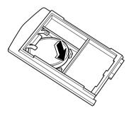
6. Align the front and back covers and snap the transmitter shut.
