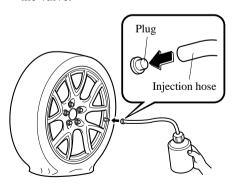
Hold the bottom of the bottle upright, squeeze the bottle with your hands, and inject the entire amount of tire sealant into the tire.
