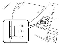
6. Pull it out again and examine the level. The level is normal if it is between Low and Full.
