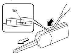
3. Insert a small flathead screwdriver into the slot and gently pry open the transmitter.
