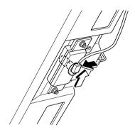
Rotate the bulb socket counterclockwise as shown in the figure and pull it out, then pull out the bulb from the socket.
