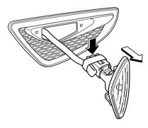
4. Replace with a new light unit and install it in the reverse order of the removal procedure.
