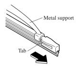
Remove the metal stiffeners from each blade rubber and install them in the new blade.
