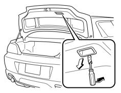
2. Disengage the pin in each clip securing the trunk trim using a (+ ) screwdriver, remove the screws and clips, and then remove the trunk trim.
