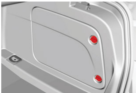
Battery Access Panel
