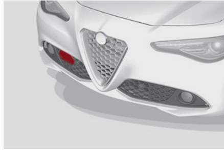
Front Bumper Radar Location
