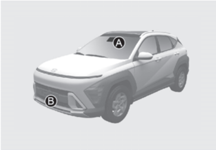
[A] Front view camera [B] Front radar
