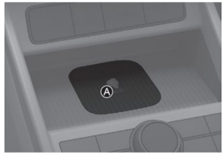
[A] Vehicle authentication pad (Wireless charging pad)
