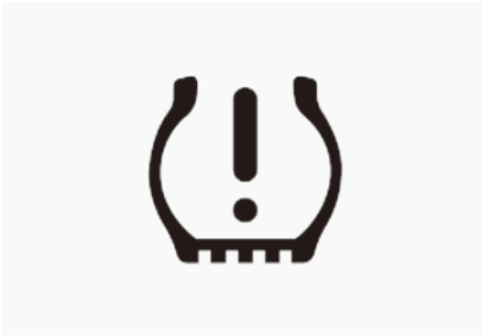
Low Tire Pressure Warning Light
