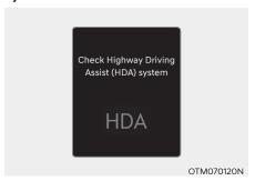
When Highway Driving Assist or Highway Lane Change function is not working properly, the 'Check Highway Driving Assist (HDA) system' warning message will appear, and the \( \frac{\Lambda}{\text{ warning light will illuminate on the cluster. We recommend that the function be inspected by an
