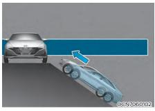
Rear Cross-Traffic Safety system may be limited when the vehicle is on a uphill or downhill slope, or near it, and may not detect the vehicle approaching from the left or right. If this occurs, the system may not warn the driver when necessary.
