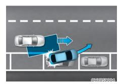
When you are driving forward out of a parking space, if the system judges that there is a collision risk with an approaching vehicle in the blind spot, the function will help avoid a collision by applying the brake.
