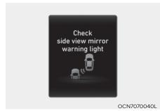
When the outside rearview mirror warning light is not working properly, the 'Check side view mirror warning light' warning message will appear on the cluster. We recommend that the system be inspected by an authorized HYUNDAI dealer.
