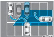
Rear Cross-Traffic Safety system may detect vehicles which are parking or pulling out near your vehicle (for example: a vehicle leaving beside your vehicle, a vehicle parking or pulling out in the rear area, a vehicle approaching your vehicle making a turn, etc.). If this occurs, the system may unnecessarily warn the driver. Always check your surroundings
