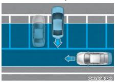
Rear Cross-Traffic Safety system may detect vehicles passing by behind you when parking in reverse into a parking space. If this occurs, the system may unnecessarily warn the driver.
