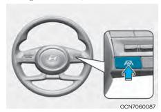
With the engine on, press and hold the Lane Driving Assist button located on the steering wheel to turn on Lane Keeping Assist. The white / indicator light will illuminate on the cluster.
