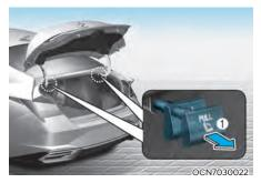
3. Pull on the seatback folding lever located in the trunk.
