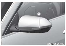
If the LED lamp (1) does not operate, have the vehicle checked by an authorized HYUNDAI dealer.
