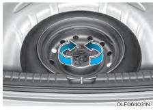
Turn the winged hold down bolt counterclockwise to remove the spare
