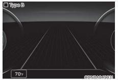
This gauge indicates the current outside air temperature by 1°F (1°C).
