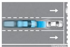
Forward Collision-Avoidance Assist is designed to help detect and monitor the vehicle ahead or help detect a pedestrian or cyclist in the roadway and warn the driver that a collision is imminent with a warning message and an audible warning, and if necessary, apply emergency braking.
