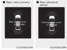
The 'Rear camera error or blockage' or 'Parking sensor error or blockage' warning message will appear on the cluster if the following situations occur:
