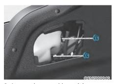
3. Loosen the assembly retaining nuts.
