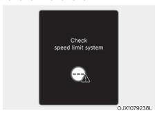
When Intelligent Speed Limit Assist is not working properly, the 'Check speed limit system' warning message will appear on the cluster. If this occurs, we recommend that the function be inspected by an authorized Hyundai dealer.
