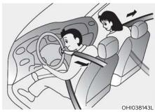
Your vehicle is equipped with driver's and front passenger's Pre-tensioner Seat Belts (Retractor Pre-tensioner). The purpose of the pre-tensioner is to make sure the seat belts fit tightly against the occupant's body in certain frontal or side collision(s).
