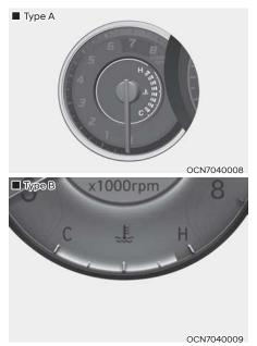
This gauge indicates the temperature of the engine coolant when the ignition switch is in the ON position.
