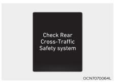
When Rear Cross-Traffic Safety system is not working properly, the 'Check Rear Cross-Traffic Safety system' warning message will appear on the cluster, and the system will turn off automatically or the system will be limited. We recommend that the system be inspected by an authorized HYUNDAI dealer.
