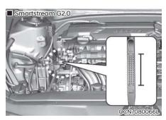
Pull the dipstick out again and check the level. The level should be between F and L.
