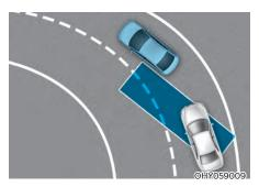
Blind-Spot Safety system may not operate properly when driving on the curved road. The system may recognize the vehicle in the same lane.
