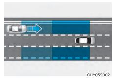
Blind-Spot Collision Assist helps detect and informs the driver that a vehicle is approaching at high speed from the blind spot area.
