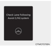
When Lane Following Assist is not working properly, the 'Check Lane Following Assist (LFA) system' warning message will appear on the cluster. If this occurs, we recommend that the function be inspected by an authorized HYUNDAI dealer.
