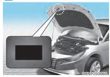
Your vehicle is filled with R-1234yf according to the regulation in your country at the time of production. You can find out which air conditioning refrigerant is applied to your vehicle on the label located inside of the hood.
