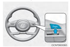
Press the Driving Assist (MODE) button to turn Manual Speed Limit Assist off. The Manual Speed Limit Assist enabled (MILMIT) indicator will go off.
