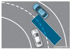
Blind-Spot Safety system may not operate properly when driving on a curved road. The system may not detect the vehicle in the next lane. Always pay attention to road and driving conditions while driving.
