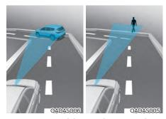
Forward Collision-Avoidance Assist may detect a vehicle or pedestrian in the next lane or outside the lane when driving on a curved road.
