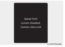
When the front windshield where the front view camera is located is covered with foreign material, such as snow or rain, it can reduce the detecting performance and temporarily limit or disable Intelligent Speed Limit Assist.
