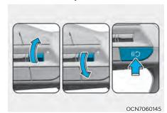
To resume Manual Speed Limit Assist after the system was paused, push the +, -, || 5 switch.
