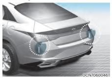
The rear corner radars are sensors located inside the rear bumper to help detect the side and rear areas. Always keep the rear bumper clean for proper operation of Safe Exit Warning.
