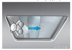
If an object or part of the body is detected while the sunroof glass is closing automatically, it will reverse the direction, and then stop.
