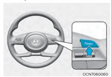
1. Press and hold Driving Assist (MODE) button at the desired speed. The Manual Speed Limit Assist enabled ((S) LIMIT) indicator will illuminate on the cluster.
