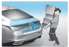
On a vehicle equipped with a smart key, the trunk can be opened using the Smart Trunk release system.
