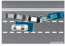
When changing lanes by detecting the lane ahead, if the system judges that there is a collision risk with an approaching vehicle in the blind spot, the function will help avoid a collision by applying the brake.
