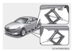
7. Place the jack at the designated jacking position under the frame closest to the tire you are changing. The jacking positions are plates welded to the frame with two notches. Never jack at any other position or part of the vehicle. Doing so may damage the side sill molding or other parts of the vehicle.
