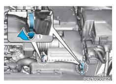
1. Loosen the air cleaner cover attaching clip (1) and open the cover.
