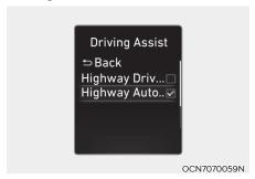
With the engine on, select 'Driver Assistance → Driving Assist → Highway Auto Speed Change' from the Settings menu to turn on Navigation-based Smart Cruise Control and deselect to turn off the system.
