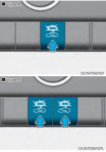
The air intake control button is used to select either Fresh mode (outside air) or Recirculation mode (cabin air).
