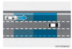
Blind-Spot Collision Warning helps detect and informs the driver that a vehicle is approaching at high speed from the blind spot area.
