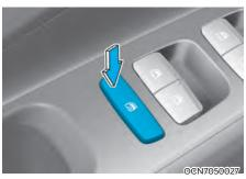
The driver can disable the power window switches on the rear passenger doors by pressing the power window lock switch.
