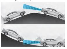
Blind-Spot Safety system may not operate properly when driving on a slope. The system may not detect the vehicle in the next lane or may incorrectly detect the ground or structure.
