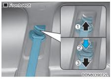
To raise the height adjuster, pull it up (1). To lower it, push it down (3) while pressing the height adjuster button (2). Release the button to lock the anchor into position. Try sliding the height adjuster to make sure that it has locked into position.
