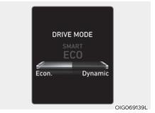
With the standard driving style in the center, the left side of the gauge is 'Econ.' and right side is 'Dynamic' style.
