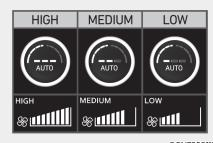
You can control the blower strength in three stages by pushing the AUTO button during automatic operation.
