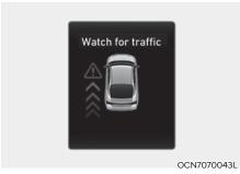
Collision warning when exiting vehicle
