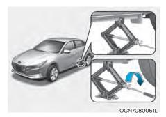
Insert the jack handle into the jack and turn it clockwise, raising the vehicle until the tire clears the ground.
