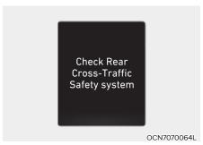
When Rear Cross-Traffic Safety system is not working properly, the 'Check Rear Cross-Traffic Safety system(s)' warning message will appear on the cluster, and the system will turn off automatically, or the system will be limited. We recommend that the system be inspected by an authorized HYUNDAI dealer.
