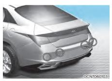
The rear ultrasonic sensors are located inside the rear bumper to detect objects in the rear area. If the sensors are covered with foreign material, such as snow or rain, it may adversely affect sensor performance and Reverse Parking Collision-Avoidance Assist may not operate normally. Always keep the rear bumper clean.
