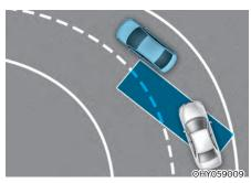
Blind-Spot Safety system may not operate properly when driving on a curved road. The system may recognize a vehicle in the same lane. Always pay attention to road and
