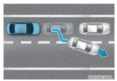
When a vehicle in front of you merges out of the lane, Smart Cruise Control may not immediately detect the new vehicle that is now in front of you.
