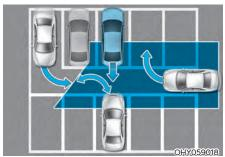
Rear Cross-Traffic Safety system may detect vehicles which are parking or pulling out near your vehicle (for example: a vehicle leaving beside your vehicle, a vehicle parking or pulling out in the rear area, a vehicle approaching your vehicle making a turn, etc.). If this occurs, the system may unnecessarily warn the driver and control the brake.
