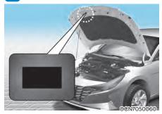
Your vehicle is filled with R-1234yf according to the regulation in your country at the time of production. You can find out which air conditioning refrigerant is applied to your vehicle on the label located in front of the engine compartment.
