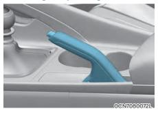
Check the stroke of the parking brake by counting the number of "clicks" heard while fully applying it from the released position. Also, the parking brake alone should securely hold the vehicle on a fairly steep grade. If the stroke is more or less than specified, we recommend that the system be serviced by an authorized HYUNDAI dealer.
