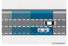
Blind-Spot Collision Warning helps detect and inform the driver that a vehicle is in the blind spot.
