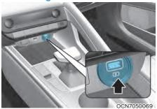
Insert the USB charger into the USB port, and re-charge a smart phone or a tablet PC.
