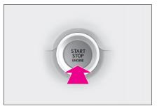
4 To stop the engine, press and hold the engine switch for 2 consecutive seconds or more, or press it briefly 3 times or more in succession.
