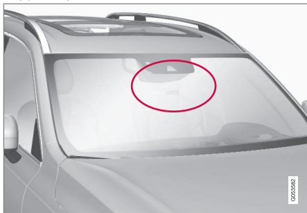
Location of radar sensor
