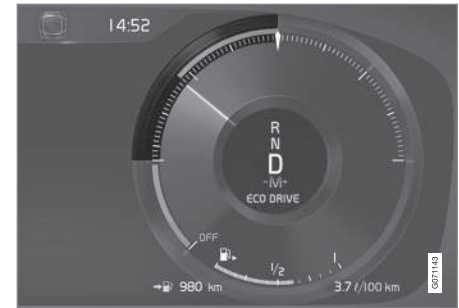
Eco gauge in 12" instrument panel*.
