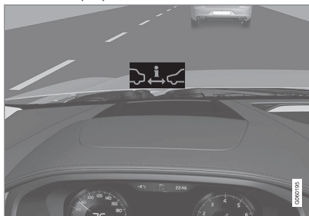
Symbol for Distance Alert on the windshield with head-up display
