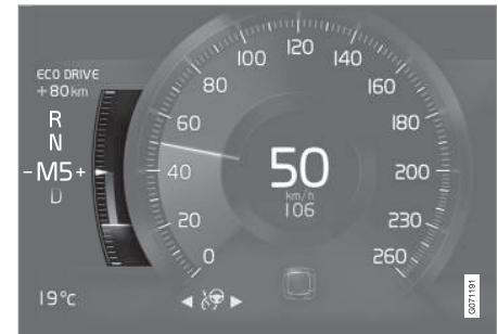
Eco gauge in 8" instrument panel.
