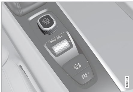
Start knob in the tunnel console.
