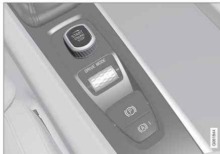
Start knob in the tunnel console.
