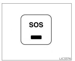
The E-call (SOS) button is used in combination with an INFINITI InTouch™ Services subscription to call for assistance in case of an emergency.
