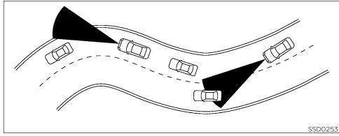
When driving on some roads, such as winding, hilly, curved, narrow roads, or roads which are under construction, the ICC sensor may detect vehicles in a different lane, or may temporarily not detect a vehicle traveling ahead. This may cause the ICC system to decelerate or accelerate the vehicle.
