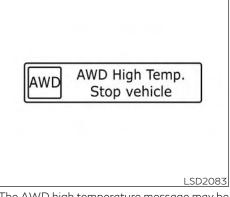
The AWD high temperature message may be displayed while trying to free a stuck vehicle due to increased oil temperature. The driving mode may change to 2-Wheel Drive (2WD). If this message is displayed, stop the vehicle with the engine idling, as soon as it is safe to do so. Then if the message turns off, you can continue drivina.
