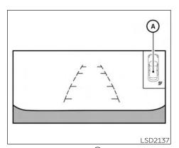
The system indicators  $\begin{tabular}{l} \textcircled{A} \end{tabular}$  will appear when the vehicle moves closer to an object.
