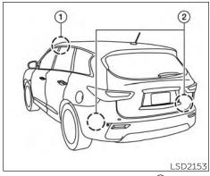
The BSI system uses a camera (1) installed behind the windshield to monitor the lane markers of your traveling lane and radar sensors (2) installed near the rear bumper to detect other vehicles in an adjacent lane.
