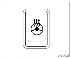
The heated steering wheel system is designed to operate only when the surface temperature of the steering wheel is below 68°F (20°C).
