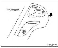
To set cruising speed, accelerate your vehicle to the desired speed, push the COAST/SET switch and release it. The ICC system set indicator (green), vehicle ahead detection indicator, set distance indicator and set vehicle speed indicator (B) will come on. Take your foot off the accelerator pedal. Your vehicle will maintain the set speed.
