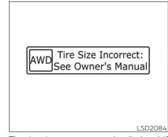
The tire size message may be displayed if there is a large difference between the diameters of front and rear wheels. Pull off the road in a safe area, with the engine idling. Check that all tire sizes are the same, that the tire pressure is correct and that the tires are not excessively worn.
