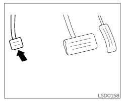
**To engage:** Firmly depress the parking brake.
