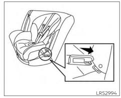
**Forward-facing rigid-mounted – step 2** positions that do not have a top tether anchor.
