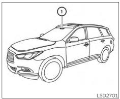
The LDW system monitors the lane markers on the traveling lane using the camera unit (1) located above the inside mirror. When the camera unit detects that the vehicle is traveling close to either the left or the right of the traveling lane, the LDW indicator in the vehicle information display blinks in orange and a warning chime sounds.
