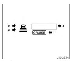
ICC (vehicle-to-vehicle distance control) mode display and indicators
