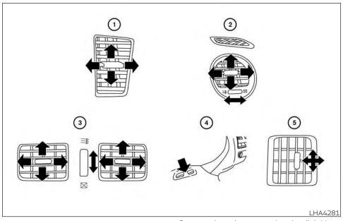
The vents underneath the first row (4) and second row seats are operational when the vi or the vi air flow mode is selected. These vents cannot be closed. For additional information, refer to "Air flow control" in this section
