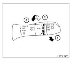
RAIN-SENSING AUTO WIPER SYSTEM (if so equipped)
