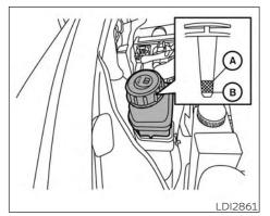
Check the fluid level in the reservoir
