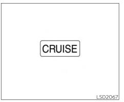
If the indicator stays on, it may indicate that the Preview Function is malfunctioning (the brake is operative). Although the vehicle is still drivable under normal conditions, have the vehicle checked. It is recommended that you visit an INFINITI retailer for this service.
