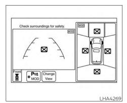
When the "[X]" icon is displayed on the screen, the camera image may be receiving temporary electronic disturbances from surrounding devices. This will not hinder normal driving operation but the system should be inspected. It is recommended that you visit an INFINITI retailer for this service
