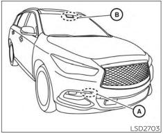
The FEB with Pedestrian Detection system uses a radar sensor (A) located behind the lower grille of the front bumper to measure the distance to the vehicle ahead in the same lane. For pedestrians, the FEB with Pedestrian Detection system uses a camera (B) installed behind the windshield in addition to the radar sensor
