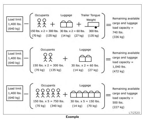
Steps for determining correct load limit
