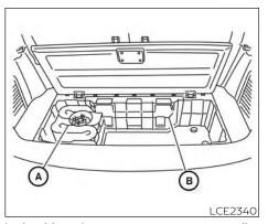
It should not be necessary to remove or dislocate the Bose® subwoofer (if so equipped) A when removing the jack and tool kit cover
