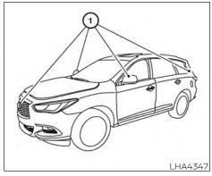
To display the multiple views, the Around View® Monitor system uses cameras located in the front grille, on the vehicle's outside mirrors and one just above the vehicle's license plate (1).
