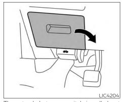
The extended storage switch is pulled out when in transit from the factory to the retailer. It is located in the fuse panel to the left of the steering wheel on the instrument panel. If any electrical equipment does not operate, ensure the extended storage switch is pushed fully in place, as shown.
