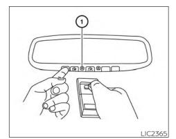
1. Position the end of your hand-held transmitter 1-3 in (2-8 cm) away from the HomeLink® surface, keeping the HomeLink® indicator light (1) in view.
