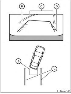
3. Slowly back up the vehicle adjusting the steering wheel so that the predicted course lines (B) enter the parking space **©**.
