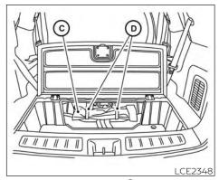
3. Remove the tool kit © by releasing the Velcro straps (**D**).
