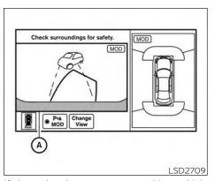
If the radar detects an approaching vehicle from the side, the system chimes a sound (single beep), the side BSW/RCTA indicator light on the side of the approaching vehicle flashes and a yellow rectangular frame appears in the display (A).
