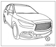
The PFCW system uses a radar sensor (A) located behind the lower grille of the front bumper to measure the distance to the vehicle ahead in the same lane.
