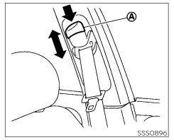
(A) Shoulder belt height adjust button Shoulder belt height adjustment (front and 2nd row outboard seats)
