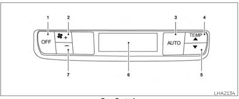
**crease buttons** Adjusts the rear fan speed up or down.
