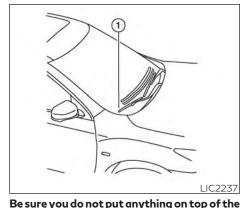
autolight sensor located in the top side ① of the instrument panel. The autolight sensor controls the autolight; if it is covered, the autolight sensor reacts as if it is dark out and the headlights will illuminate. If this occurs while parked with the engine off and the ignition switch placed in the ON position, your vehicle's battery could become discharged.
