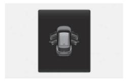
This warning appears if any door or hood or liftgate is left open. The warning indicates which door is open on the cluster display.
