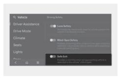
With the engine on, select **Setup > Vehicle > Driver Assistance > Driving Safety** > **Safe Exit** from the Settings menu to turn on Safe Exit Warning and deselect to turn off the function.
