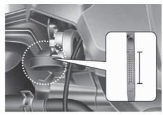
7. If the oil level is below the L, add enough oil to bring the level to F.
