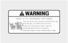
Airbag warning labels, required by the U.S. National Highway Traffic Safety Administration (NHTSA), are attached to alert the driver and passengers of potential risks of the airbag system. Be sure to read all of the information about the airbags that are installed on your vehicle in this Owners Manual.
