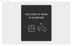
When Highway Driving Assist is operating, your vehicle will stop if the vehicle ahead of you stops. Also, if the vehicle ahead of you starts moving within 30 seconds after the stop, your vehicle will start as well. In addition, after the vehicle has stopped and 30 seconds have passed, the "Use switch or pedal to accelerate" message will appear on the instrument cluster. Depress the accelerator pedal or operate the + switch, - switch or IIO switch to start driving.
