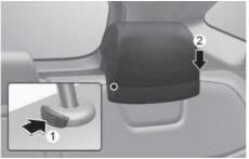
3. Locate the seatbelt toward the outboard position before folding down the seatback to avoid the seatbelt system interfering with the seatback.
