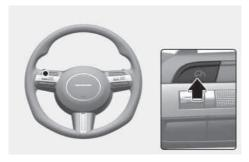
Press the Driving Assist (ਨ) button to turn Manual Speed Limit Assist off. The Speed Limit (ਿਯੋ⊔ਅਸ) indicator will go off.
