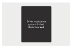
When the rear bumper around the rear corner radar or sensor is covered with foreign material, such as snow or rain, or installing a trailer or carrier, it can reduce the detecting performance and temporarily limit or disable Blind-Spot Collision-Avoidance Assist.
