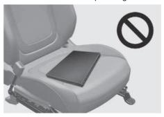
Make sure the seat has been completely dried before driving the vehicle. If large quantity of liquid has been spilled on the front passenger seat, the airbag warning light may illuminate or malfunction.
