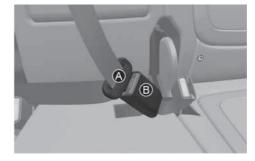
Insert the tongue plate (A) into the buckle (B) until an audible "click" is heard, indicating the latch is locked. Pull the shoulder portion of the belt to snug the belt across your hips and remove slack. Make sure the seat belt is not twisted. When using the rear center seat belt, use the buckle with the "CENTER" mark.
