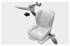
4. Slowly allow the shoulder portion of the seat belt to retract and listen for an audible "clicking" or "ratcheting" sound. This indicates that the retractor is in the Automatic Locking mode. If no distinct sound is heard, repeat Step 3 and 4.
