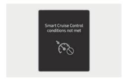
If the Driving Assist button, + switch, - switch or IIO switch is operated when Smart Cruise Control operating conditions are not satisfied, the "Smart Cruise Ctrl. conditions not met" will appear on the instrument cluster, and an audible warning will sound.
