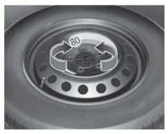
Turn the winged hold down bolt counterclockwise to remove the spare tire. Store the spare tire in the same compartment by turning the winged hold down bolt clockwise.
