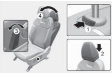
To reinstall the head restraint:
