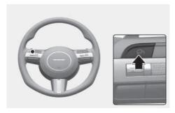
To turn Smart Cruise Control off, press the Driving Assist (た) button.
