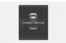
When an approaching vehicle from the rear is detected at the moment a door is opened, the "Collision Warning" warning message will appear on the instrument cluster, and an audible warning will sound.  Safe Exit Warning will warn the driver when your vehicle speed is below 2 mph (3 km/h), and the speed of the approaching vehicle from the rear is above 4 mph (6 km/h).
