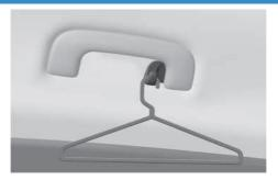
Only hang soft clothing without heavy, sharp or breakable objects in the clothes pockets. In a collision or when the curtain airbag is inflated, the objects could move and cause serious injury.
