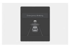
To warn the driver that emergency braking will be assisted, Forward Safety warning light (♣) blinking, the "Emergency Braking" warning message will appear on the cluster, an audible warning will sound, and the steering wheel will vibrate.
