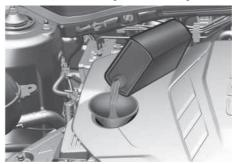
Use only the specified engine oil (Refer to the "Recommended lubricants and capacities" section in chapter 10).
