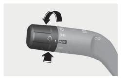
High Beam Assist automatically adjusts the headlights between high beam and low beam depending on the light detected from oncoming vehicles or vehicles in front using the front view camera.
