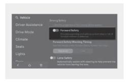
With the engine on, select **Setup** > **Vehicle** > **Driver Assistance** > **Driving Safety** in the infotainment system to set whether to use each function.
