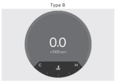
The engine coolant temperature gauge indicates the temperature of the engine coolant when the Engine Start/Stop button is in the ON position.
