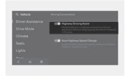
With the engine on, select or deselect Setup > Vehicle > Driver Assistance > Driving Convenience > Highway Driving Assist from the infotainment system to set whether to use each function.
