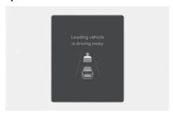
When a detected vehicle in front departs from a stop, Leading Vehicle Departure Alert will inform the driver by displaying the "Leading vehicle is driving away" message on the instrument cluster and an audible warning will sound.
