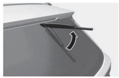
3. Press the wiper blade slot (1). Then remove the wiper blade (2).
