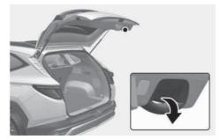
Lower the liftgate lid and press down until it locks. Always check it is secure by pulling on the handle.
