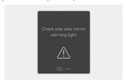
When the side view mirror warning light is not working properly, the "Check side view mirror warning light" warning message will appear on the instrument cluster for several seconds, and the master warning light (A) will appear on the instrument cluster. If this occurs, have your vehicle inspected by an authorized HYUNDAI dealer.
