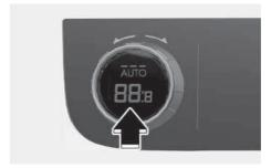
You can control the fan speed in three stages by pressing the **AUTO** button during automatic operation.
