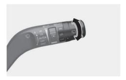
The rear wiper operates while the vehicle is in reverse with the front wiper on. You can select the function from the Settings menu in the infotainment system. Select:
