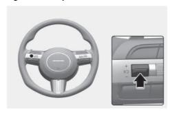
Press the IIO switch to temporarily pause the set speed limit. The set speed limit will turn off but the Speed Limit (©LIMIT) indicator will stay on.
