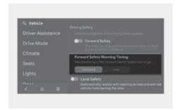
With the Engine Start/Stop button ON, select **Setup > Vehicle > Driver Assistance > Driving Safety > Forward Safety Warning Timing** from the Settings menu to change the initial warning activation time. Warning Timing is set to **Standard** at the factory.
