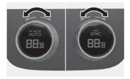
The temperature increases by turning the knob to the right (red side). The temperature decreases by turning the knob to the left (blue side).
