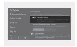
With the engine on, select **Setup > Vehicle > Driver Assistance > Driving Safety** from the settings menu in the infotainment system to set whether to use each function.
