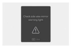
When the side view mirror warning light is not working properly, the "Check side view mirror warning light" warning message will appear on the instrument cluster for several seconds, and the master (A) warning light will illuminate on the instrument cluster. If this occurs, have your vehicle inspected by an authorized HYUNDAI dealer.
