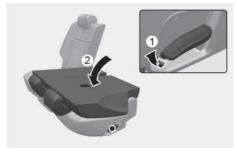
5. Lift and push the seatback rearward while lifting up the front portion of the folding lever.
