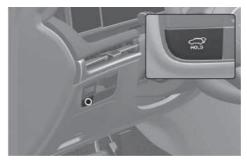
When the liftgate is closed, press the power liftgate open/close button for 1 second. The power liftgate opens with a warning sound.
