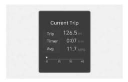
The trip computer mode displays information related to vehicle driving parameters including fuel economy, tripmeter information, and vehicle speed. Current trip is initialized when the vehicle is turned off and the driver's door is open, or when the vehicle is turned on 3 minutes after the vehicle is turned off.
