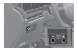
When the vehicle's parking lights or headlights are on, press the illumination control switch to adjust the brightness of the instrument panel illumination. When pressing the illumination control switch, the interior switch illumination intensity is also adjusted.
