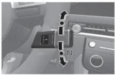
To shift the gear to N (Neutral), rotate the rotary gear shift dial to N (Neutral) from R (Reverse) or D (Drive) while depressing the brake pedal.
