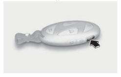
When the liftgate is closed, press the power liftgate open button for 1 second. The liftgate will open with a warning sound.
