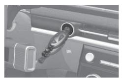
If the smart key is in close proximity to your mobile phone, the signal could be blocked by your mobile phone's operational signals. This is specifically relevant when the phone is active such as making and receiving calls, text messaging, and/or sending/receiving emails. If possible, avoid keeping the smart key and your mobile phone in the same location such as pants or jacket pocket to avoid interference between the two devices.
