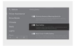
With the engine on, select or deselect **Setup > Vehicle > Driver Assistance > Parking Safety** in the infotainment system to set whether to use each function.
