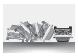
Front airbags may not inflate in rollover crash because front airbag deployment would not provide additional occupant protection.
