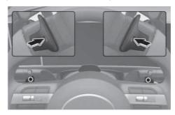
The paddle shifter is available when the shift lever/dial is in the D (Drive) position or the manual shift mode.
