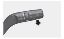
In the OFF position, pull the lever gently toward you to spray washer fluid on the windshield and to run the wipers 1-3 cycles. The spray and wiper operation continues until you release the lever. If the washer does not work, you may need to add washer fluid to the washer fluid reservoir.
