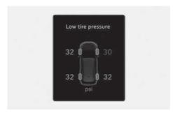
This warning message appears if the tire pressure is low. The corresponding tire on the vehicle is illuminated.
