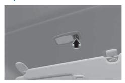
Push the switch to turn the lamp on or off.
