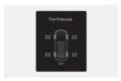
• You can check the tire pressure in the utility view mode in the cluster display. Refer to the "View modes" section in chapter 4.
