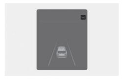
If the vehicle ahead and/or both lane markings are detected and your vehicle speed is below 110 mph (180 km/h), the green  $(\Theta)$  indicator light appears on the cluster, and Lane Following Assist helps center the vehicle in the lane by assisting the steering wheel.
