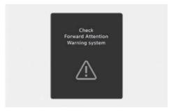
When Forward Attention Warning is not working properly, the "Check Forward Attention Warning system" warning message will appear on the cluster. If this occurs, have the vehicle inspected by an authorized HYUNDAI dealer.
