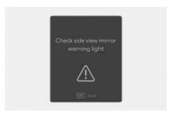
When the side view mirror warning light is not working properly, the "Check side view mirror warning light" warning message appears on the instrument cluster for several seconds, and the master  $(\triangle)$  warning light illuminates on the
