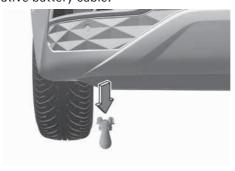
Loosen the retaining clips under the bumper and screws on the wheel house trim. 3. Prey trim under the bumper toward the vehicle.
