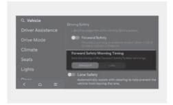
With the vehicle on, select **Setup** > **Vehicle** > **Driver Assistance** > **Driving Safety** > **Forward Safety Warning Timing** settings menu in the infotainment system to change the initial warning activation time for Forward Collision-Avoidance Assist. The warning time can be set to either **Standard** or **Late**.
