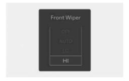
This indicator displays which wiper speed is selected using the wiper control. You can activate or deactivate Wiper/Lights display function from the Settings menu in the infotainment system. Select:
