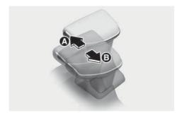
[A] Push the lever forwards once to shift up one gear.
