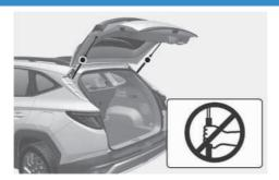
Always close the liftgate before driving. Do not grab or hold on to the liftgate support struts or they may be damaged. Deformation of the liftgate support struts may result in vehicle damage and personal injury.
