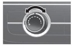
Turn the knob to the right to increase the fan speed and airflow. Turn the knob to the left to decrease fan speed and airflow.
