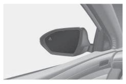
When the vehicle is detected in the rear left and right lanes, to warn the driver a vehicle is detected, the warning light on the side view mirror and Head-Up-Display (if equipped) will illuminates. Vehicle detection operates under following conditions.
