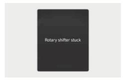
This message appears when the rotary gear shift dial does not return back to it's normal position after rotating it.
