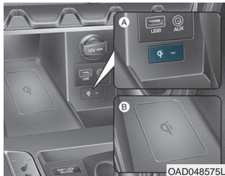
[A]: Indicator light, [B]: Charging pad
