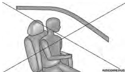
Not Seated Properly
