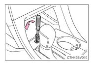
5 Press and hold the shift lock override button and then push the button on the shift knob.
