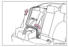
6 If the child restraint has a top tether strap, the top tether strap should be latched onto the top tether strap anchor. (→P. 67)
