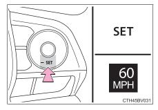
If the switch is operated while the vehicle speed is below approximately 30 mph (50 km/h) and a preceding vehicle is present, the set speed will be adjusted to approximately 30 mph (50 km/h).
