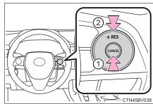
2 Pressing the "+ RES" switch resumes the cruise control and returns vehicle speed to the set speed.
