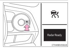
If the cruise control main switch is pressed and held for 1.5 seconds or more, the system turns on in constant speed control mode. (→P. 257)
