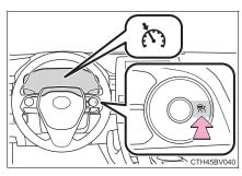
Switching to constant speed control mode is only possible when operating the switch with the cruise control off.
