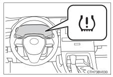
B Drive straight (with occasional left and right turns) at approximately 25 mph (40 km/h) or more for approximately 10 to 30 minutes.
