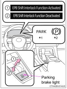
Turns automatic mode off (while the vehicle is stopped, press and hold the parking brake switch until a message is shown on the multi-information display)
