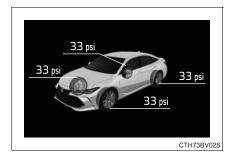
• If the tire pressure drops below a predetermined level, the driver is warned by a screen display and a warning light. (→P. 434)
