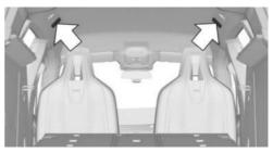
3. Insert each of the two top retaining pins of the cargo area partition net into the receptacles until they reach the stop, arrows 1, and push them forward. Make sure that the belt adjusters for the bottom hooks point forward.
