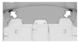
Insert each of the two top retaining pins of the cargo area partition net into the receptacles until they reach the stop, arrows 1, and push them forward.
