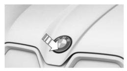
To open the container, press on the lower edge of the badge on the hood. The lid opens when the vehicle is unlocked.
