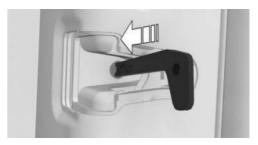
Pull the door handles to make sure they are locked. If necessary, repeat the process.
