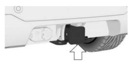
The mount for the trailer hitch is located on the rear of the vehicle, see arrow.
