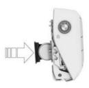
6. Insert the cover into the vehicle key.
