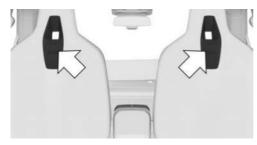
The mounts for attaching optional accessories are located behind the marked covers.
