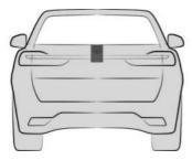
The Rear View Camera is located in the badge on the rear of the vehicle.
