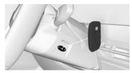
It is not possible to switch on the drive-ready state if the vehicle key has not been detected.
