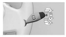
Turn the outer switch upward.
