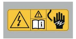
These icons found on parts of the vehicle indicate that incorrect use of high-voltage technology or of orange-colored high-voltage components poses a risk of life-threatening injury by electric shock.
