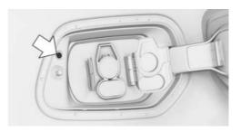
The charging cable release button is located next to the high-voltage charging socket.
