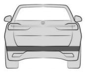
The ultrasonic sensors of the parking assistance systems are located in the rear bumper.
