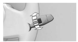
Turn the knurled wheel to adjust the sensitivity of the rain sensor.
