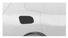
The charging socket flap is located in the rear on the right side of the vehicle.
