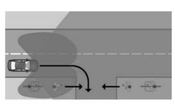
Sensors detect the traffic situation in their detection range when turning.
