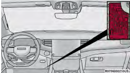
Interior Power Distribution Center Location
