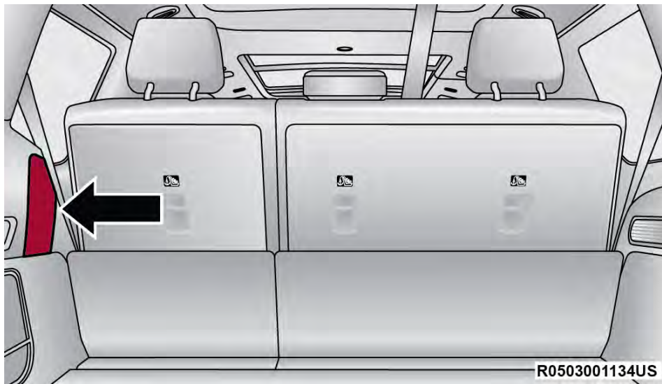
Rear Power Distribution Center Location
