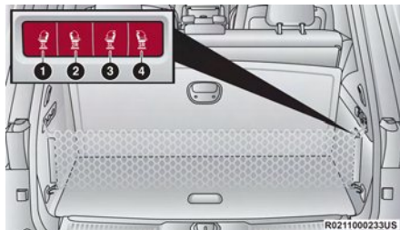
Rear Panel Power Switch Bank
