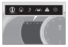
Selecting a menu icon displays a variety of vehicle data or allows vehicle settings to be customized.
