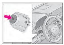
Press the Automatic High Beam switch.
