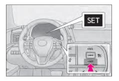
1 With the cruise control off, press and hold the cruise control main switch for 1.5 seconds or more.
