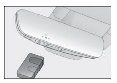
Point the remote control transmitter for the device at the rear view mirror, 1 to 3 in. (25 to 75 mm) from the HomeLink<sup>®</sup> buttons.
