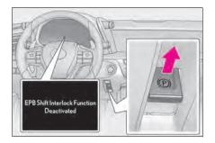
While the vehicle is stopped, pull and hold the parking brake switch until a message is shown on the multi-information display
