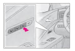
**3** Press one of the buttons for the driving position you want to recall until the buzzer sounds.
