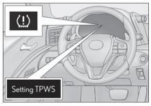
A message is displayed on the multi-information display. Also, "--" is displayed for inflation pressure of each tire on the multiinformation display while the tire pressure warning system determines the position.
