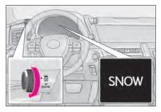
Snow mode can be selected to suit the conditions when driving on slippery road surfaces, such as on snow.
