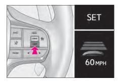
1 Press the cruise control main switch to activate the cruise control.
