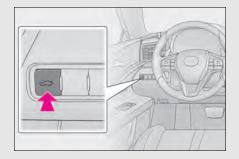
Unlock the doors, and press the trunk opener switch.
