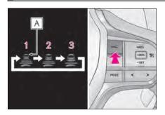
Pressing the switch changes the vehicle-to-vehicle distance as follows:
