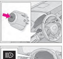
1 Press the Automatic High Beam switch.
