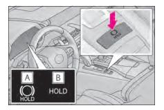
Turns the brake hold system on
