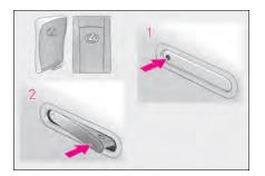
Push the depression on the front edge of the driver's door handle to unlock the door. Push the depression on the front edge of the passenger's door handle to unlock both side doors.\*
