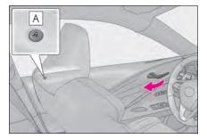
Pull the inside door handle to unlock the door.
