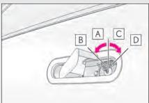
2 Insert the mechanical key while pulling on the driver's door handle.
