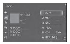
2 Select and hold "(Hold Edit)". To change the preset station to a different one, select and hold the preset station.
