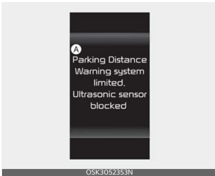
A: Parking Distance Warning system limited. Ultrasonic sensor blocked
