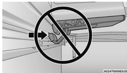
Improper Clamp Position
