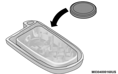
Key Fob Battery Replacement
