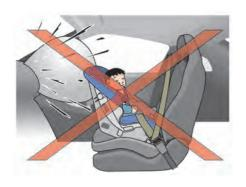
Child restraints for infants must be used in the rear-facing direction and therefore must not be used in the front seat. Position the child restraint on the seat. Always follow the restraint manufacturer's instructions.
