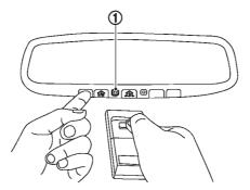
2. Using both hands, simultaneously press and hold the desired HomeLink® button and handheld transmitter button. DO NOT release until the HomeLink® indicator light ① flashes slowly and then rapidly. When the indicator light flashes rapidly, both buttons may be released. (The rapid flashing indicates successful programming.)
