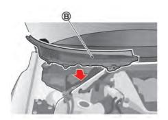
3. Unfasten the 3 clips and remove the cowl top cover ® by pulling it towards the front of the vehicle.
