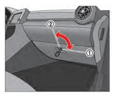
Use the mechanical key to lock 1 and unlock ② the glove box. ( 🌠 "Mechanical key" page 3-3)
