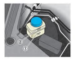
Check the fluid level in the reservoir. If the fluid is below the MIN line ① or the brake warning light comes on, add Genuine NISSAN Brake Fluid R35 Special II fluid (or equivalent) up to the MAX line (2). If fluid must be added frequently, the system should be checked. It is recommended you contact a GT-R certified NISSAN dealer.
