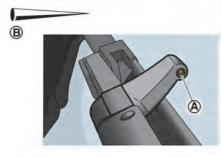
Be careful not to clog the washer nozzle ⓐ. This may cause improper windshield washer operation. If the nozzle is clogged, remove any objects with a needle or small pin ⑤. Be careful not to damage the nozzle.
