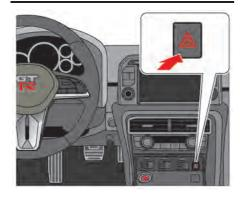
Push the switch on to warn other drivers when you must stop or park under emergency conditions. All turn signal lights will flash.
