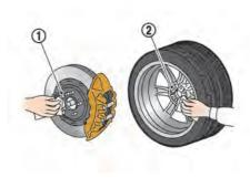
5. Remove the wheel nuts and then remove the wheel.
