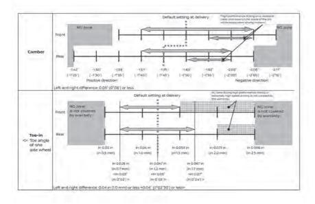
Toe-out can cause uneven tire wear or damage to areas inside the tires due to high heat. Be sure to have the wheel alignment toe-in setting checked and adjusted by your GT-R certified NISSAN dealer before any performance driving on closed circuit tracks. Obey all traffic laws when on public roads.
