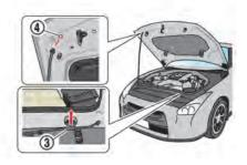
3. Grasp the insulated part of the stay ③ and release it from the hook, then securely insert it into the hood hole @.
