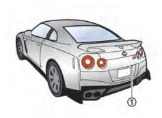
To display the rear view, the RearView Monitor system uses a camera (1) located just above the vehicle's license plate.
