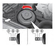
NISSAN recommends to adjust the engine oil level ① to be 0.39 in (10 mm) (1/8 gal (0.5 liters)) ② below the H mark on the engine oil dipstick. (③ range is 1.18 in (30 mm).) Before checking the oil level, run the engine until it reaches operating temperature and wait at least 5 minutes after turning off the engine. Make sure the oil level always remains above the L mark.
