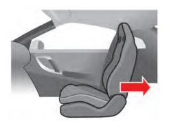
Forward-facing (front passenger seat) — step 1 Refer to all Warnings and Cautions in the "Child safety" and "Child restraints" sections before installing a child restraint.
