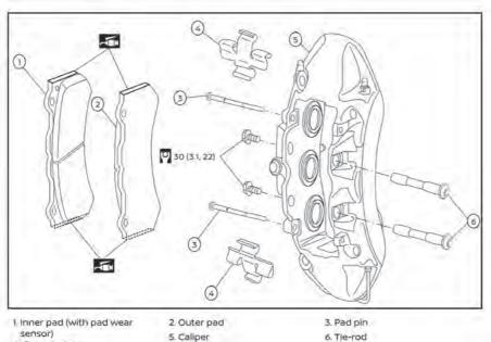
Apply MOLYKOTE 7439 or equivalent to the match face (a) of the brake pad (1)
