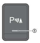
The sonar system OFF switch on the lower side of the instrument panel allows the driver to turn the sonar system on and off. To turn the sonar system on and off, the ignition switch must be in the ON position. The indicator light (1) on the switch will turn off when the system is turned off. If the indicator light flashes it may indicate a malfunction in the sonar svstem.
