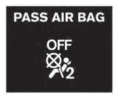
7. If the booster seat is installed in the front passenger seat, push the ignition switch to the ON position. The front passenger air bag status light may or may not illuminate depending on the size of the child and the type of booster seat used. (译 "Front passenger air bag and status light" page 1-42)
