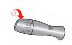
the daytime running light will remain on. Turning the switch to the position: Headlights will come on and all the other lights remain on. The daytime running light will turn off.
