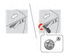
2. With the outside door handle lifted up, use the mechanical key and turn the key cylinder cap (A) counterclockwise to remove.
