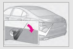
Turn the mechanical key clockwise to open.
