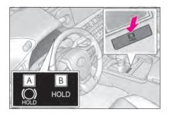
Turns the brake hold system on
