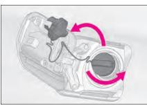
2 Turn the fuel tank cap slowly and remove it, then hang it on the back of the fuel filler door.
