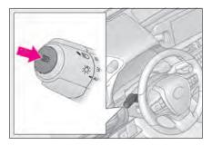
1 Press the Automatic High Beam switch.
